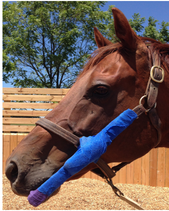
Figure 4.3: Attaching the recording device to the side of the halter allowed the audio recordings for Horse #1 to be recorded. During the recordings, the recorder moved slightly with the movement of the halter.
