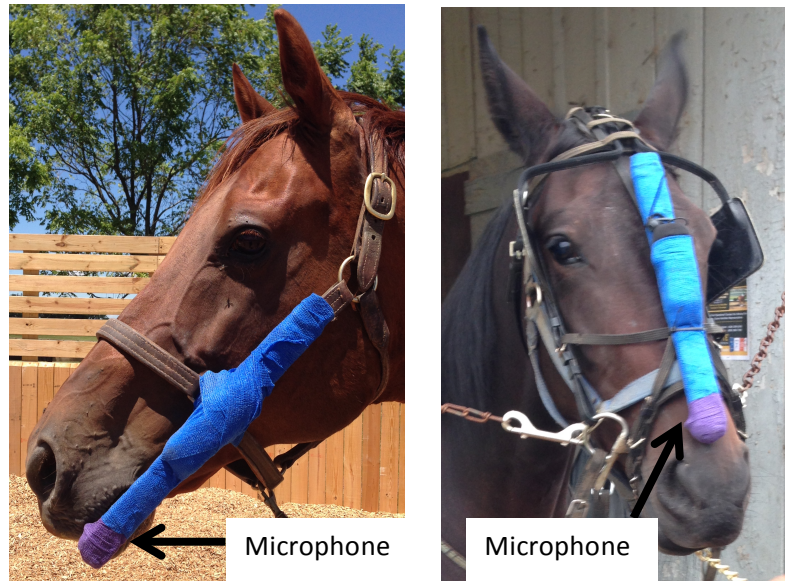
Figure 3.2: The recording device was created with wooden shims and vet wrap and attached to either the side or front of the horse's tack using zip ties to hold it firmly in place. The microphone placement was consistent for each individual horse throughout the study.
