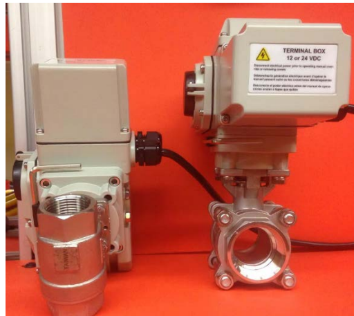
Figure 5.8 Ball valves used for supplying water to sprays on the shearer drum and impingement screen.
