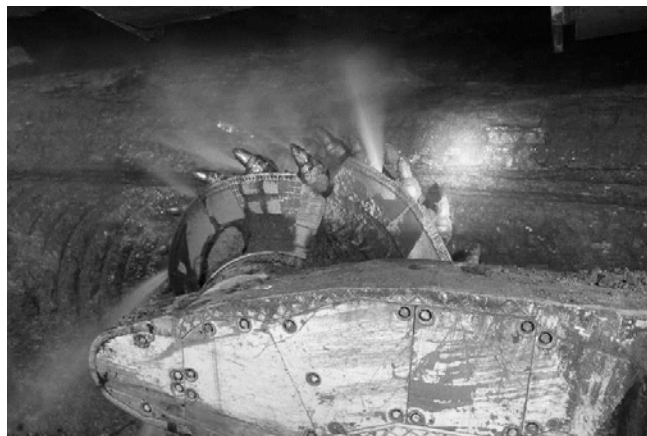
Figure 2.5. Water sprays in action (Source: Andrez Drum, Mining Tribune, Poland)
