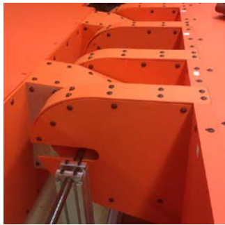
Figure 5.6 Testing the coupling of the ranging arm as well as the drive unit of the shearer.
