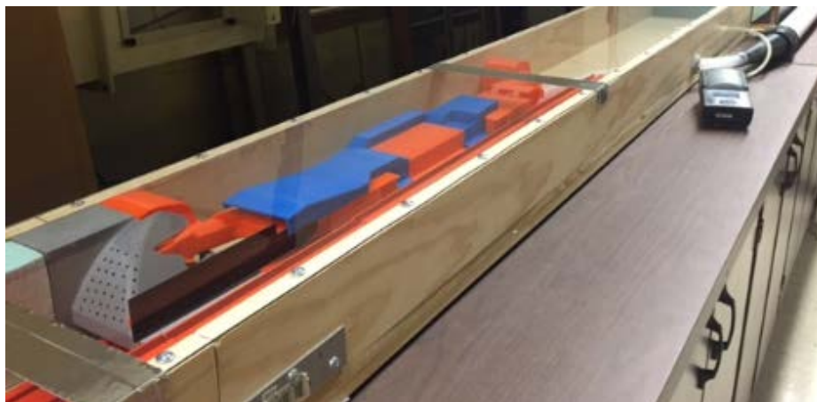
Figure 5.14 Experimental set up to measure the capture efficiency on the 1:20 scaled model.
