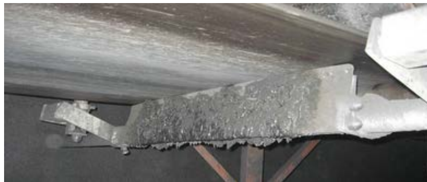
Figure 2.8 A typical coal cleaner installed underneath the belt (Source: Luoyang Ruita Rubber Co. Ltd).
