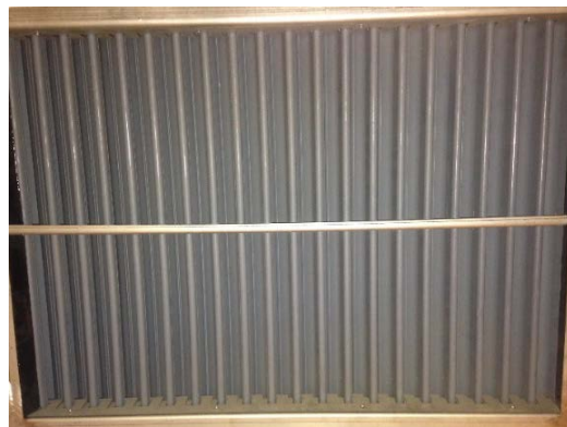
Figure 3.5 The demister to arrest the water droplets from the air.
