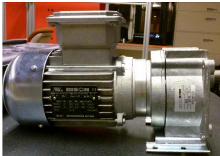
Figure 5.7 A 0.25 hp motor used to rotate the drum.
