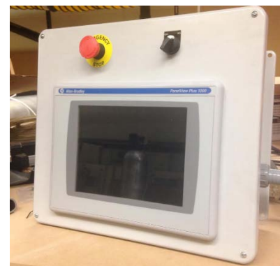
Figure 5.11 Programmable logic controllers to monitor vital parameters on the shearer, a HMI connected to the controls using an umbilical cord displays the parameters.
