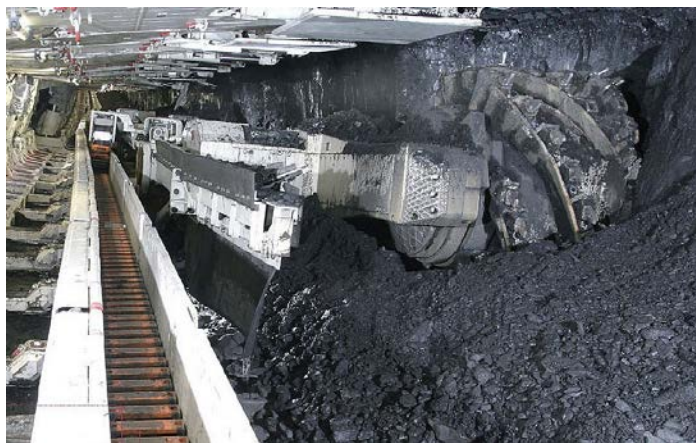
Figure 2.6. Shearer clearer on a shearer (Source: Connexa product brochure, www.connexa.com.au )
