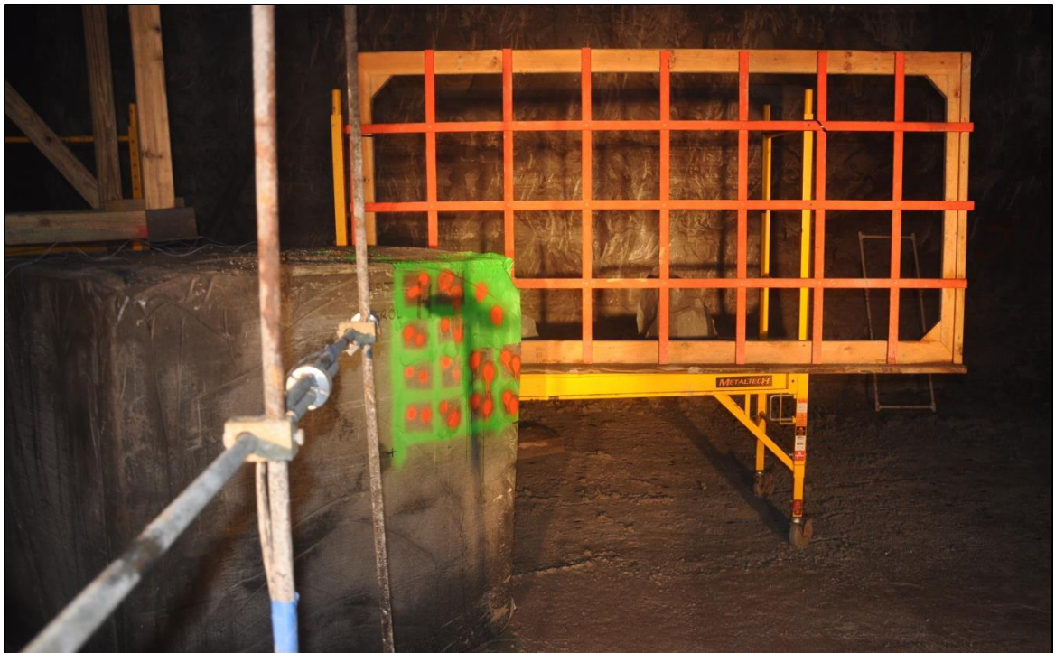
Figure 7.2: Velocity screen position for block testing
