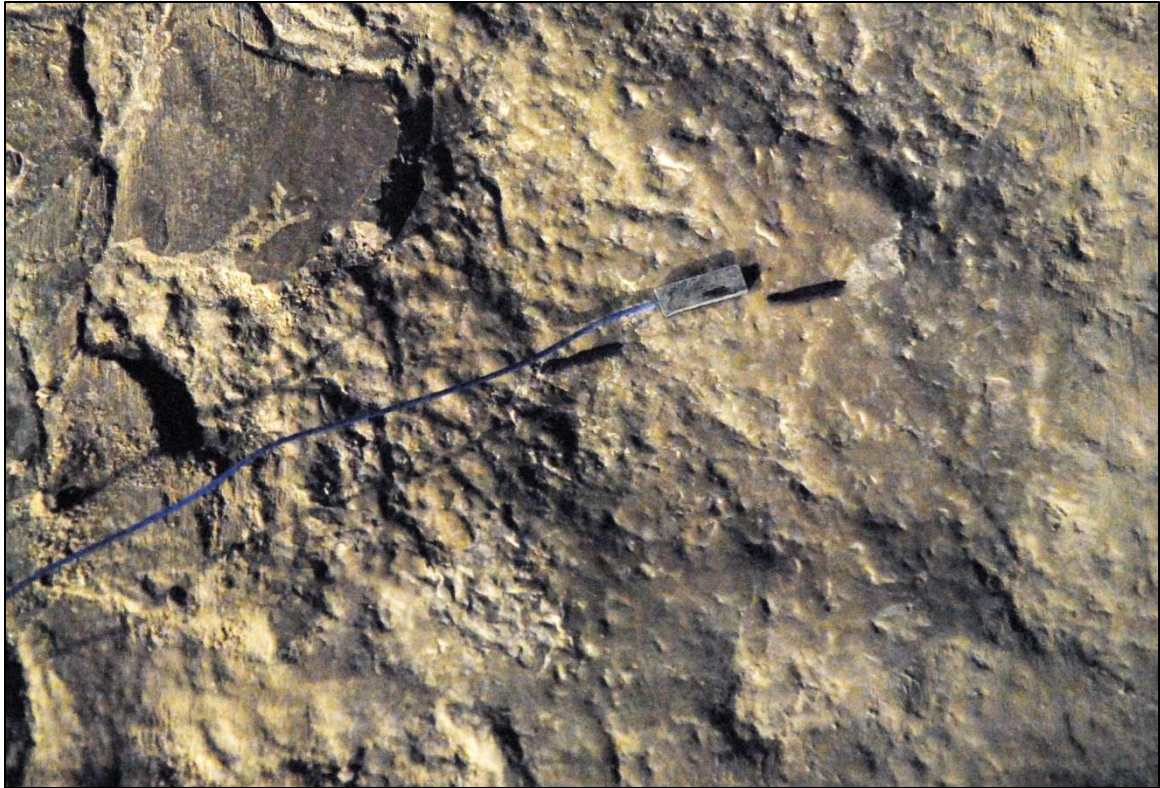
Figure 4.3: PCB strain sensor adhered to the rock surface
