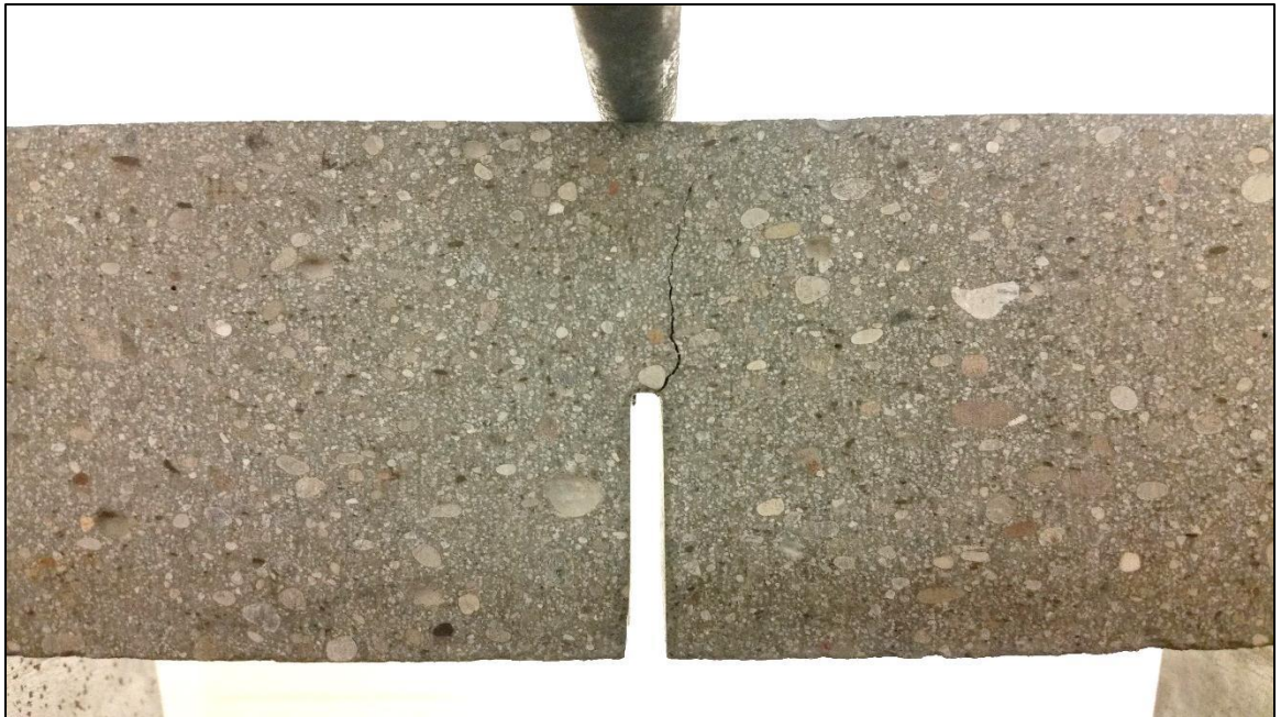
Figure 7.11: Sample beam with fracture extending from starter notch
