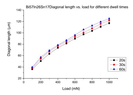
Figure 20: Dependence of the imprint diagonal length on different indentation load
