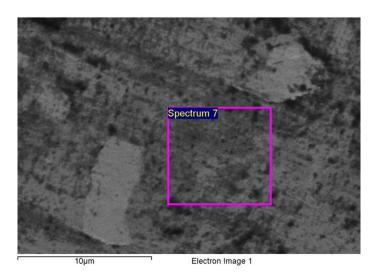
Figure 13: SEM image of Bi57In26Sn17 lead-free alloy
