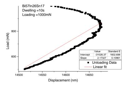
Figure 12: Unloading data without the data mask
