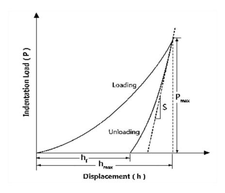
Figure 3: A typical load-displacement curve
