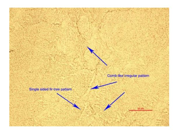
Figure 16: Optical micrograph of Bi57In26Sn17 after annealing for 9 hours at 50 °C, M=20, unit length: 50 micrometer
