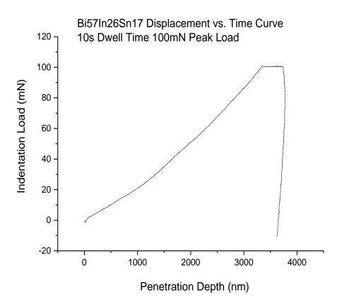
Figure 10: A typical loading-unloading curve
