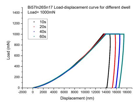
Figure 19: 3-stage loading-dwelling-unloading curves (b)
