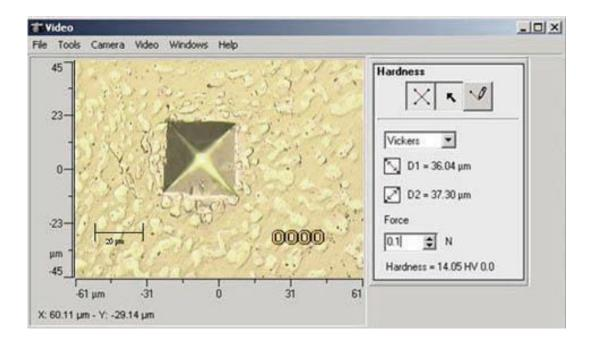
Figure 9: Measurement of the diagonal length
