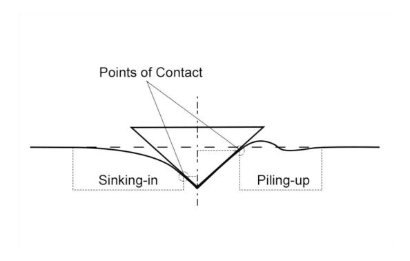
Figure 4: Schematic of sink-in and pile-up on a sample surface
