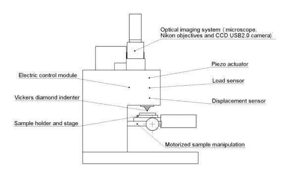
Figure 1: Schematic illustration of a micro hardness indenter
