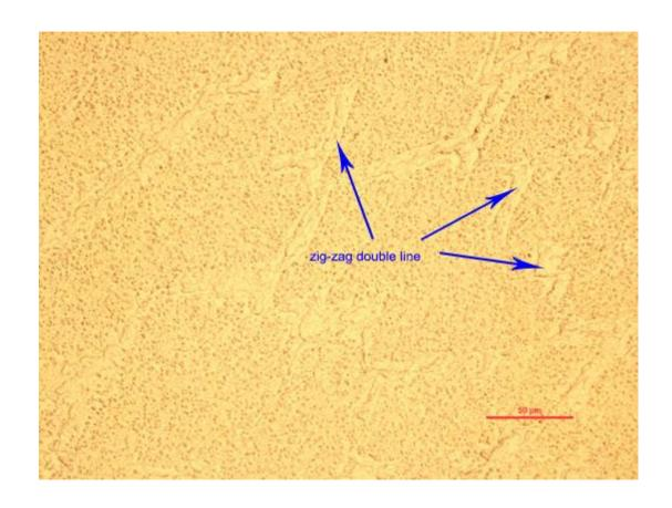
Figure 15: Optical micrograph of Bi57In26Sn17, M = 20, unit length: 50 micrometer
