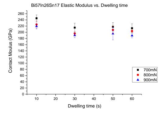
Figure 26: Time dependence of contact modulus for different indentation loads
