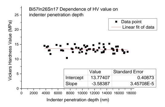
Figure 23: Dependence of Vickers hardness on the indenter penetration depth with linear fitting result
