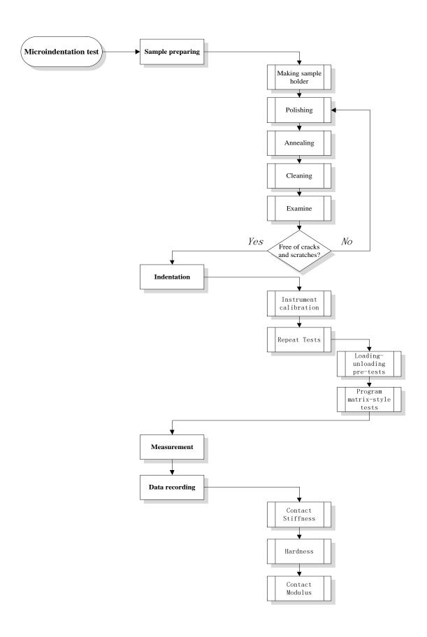
Figure 6: Experimental flow chart for the indentation of the Bi57In26Sn17 lead-free sample alloy
