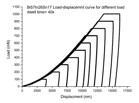
Figure 18: 3-stage loading-dwelling-unloading curves (a)
