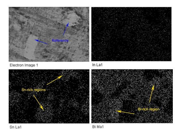
Figure 14: A group of the element maps obtained from EDX analysis
