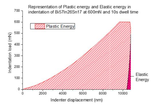
Figure 27: Representation of plastic energy and elastic energy in a typical 3-stage curve
