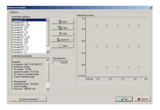
Figure 8: Indentation preset panel for a matrix test
