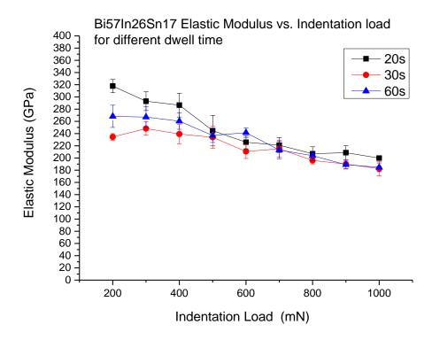
Figure 25: Load dependence of contact modulus for different dwell times
