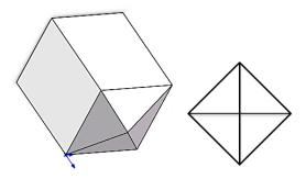
Figure 2: 3D view and top view of the Vickers hardness indenter tip
