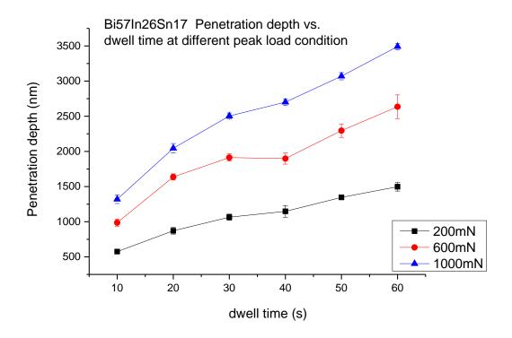
Figure 21: Dependence of the penetration depth on dwell times for different indentation peak loads
