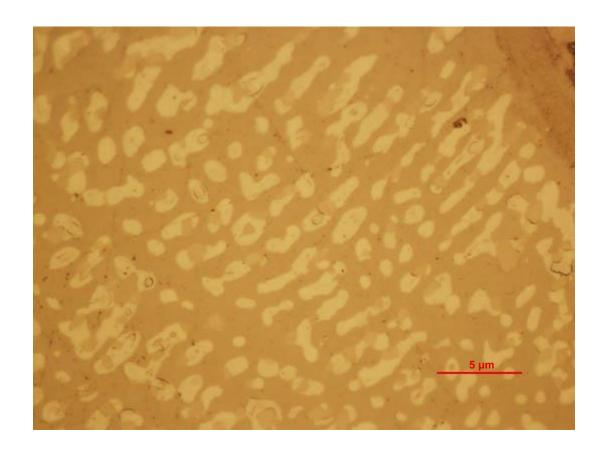
Figure 17: An enlarged view of the optical micrograph of Bi57In26Sn17 after annealing for 9 hours at 50 °C, M=200, unit length: 5 micrometer
