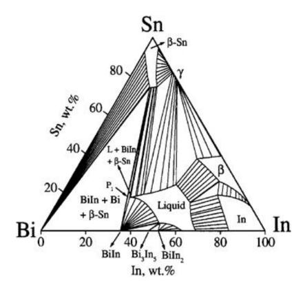
Figure 5: Isothermal phase diagram, temperature slightly below 77.9 °C
