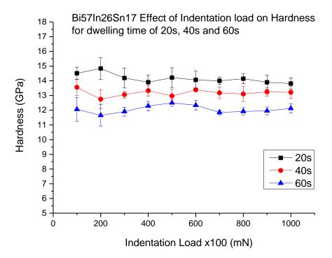
Figure 24: Vickers hardness value versus indentation load
