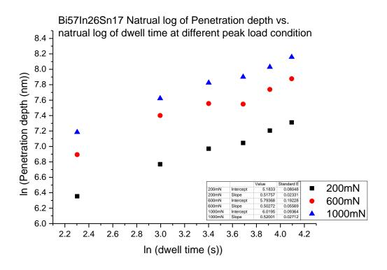
Figure 22: Dependence of the penetration depth on dwell time for different indentation peak loads in ln-ln plot
