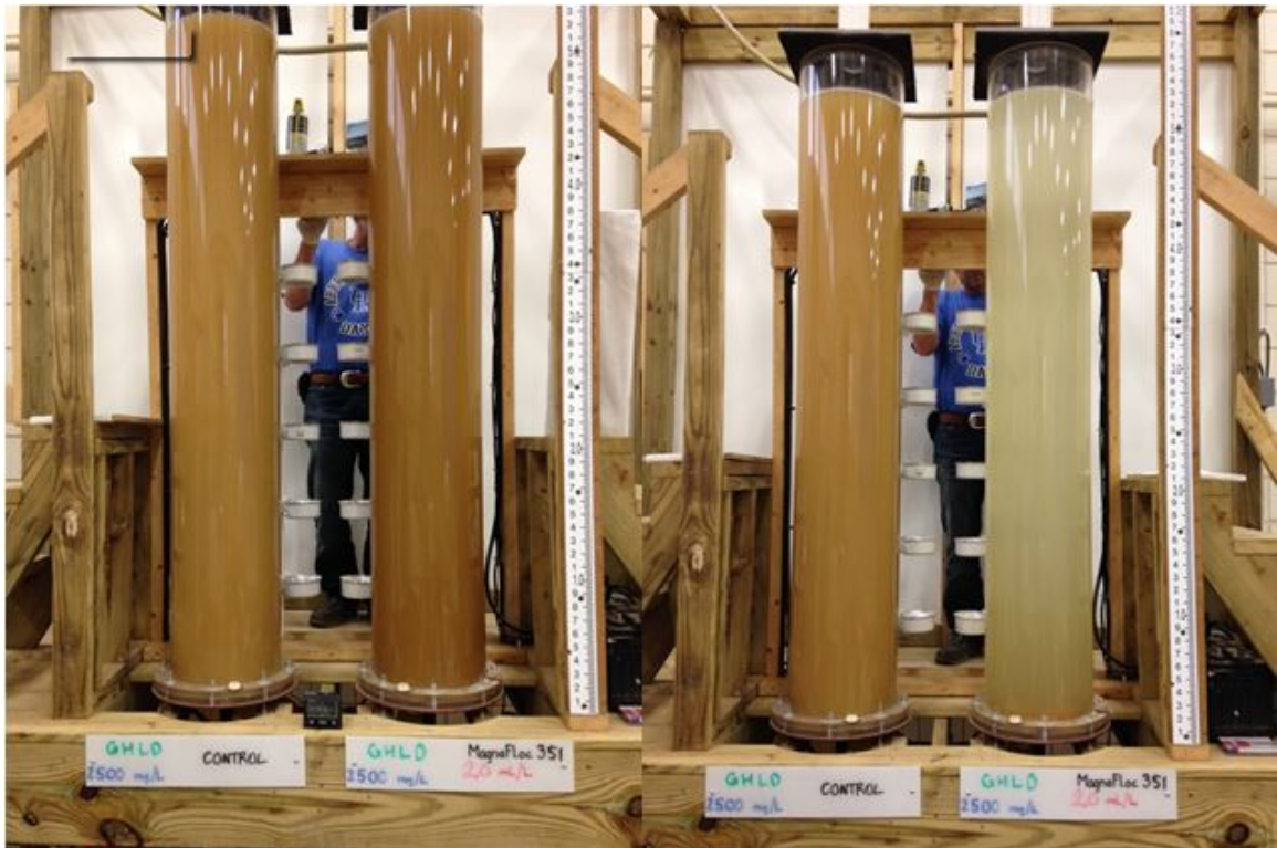
Figure 3.7: Column Comparison at 2,500 mg/L Initial Concentration at Time=0 min (left) and Time=5 min (right)
