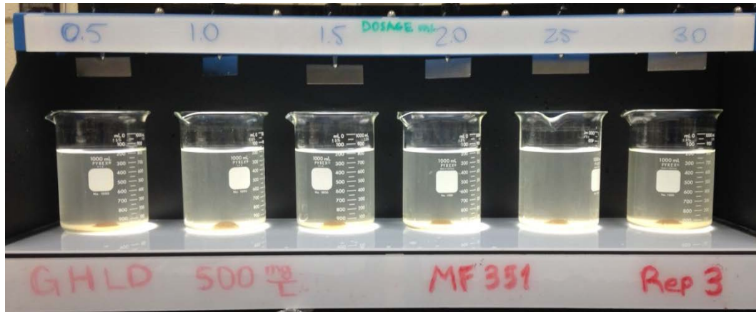
Figure 2.5: Visual Results of MF 351 at 500 mg/L Initial Concentration after 10 Minutes Settling
