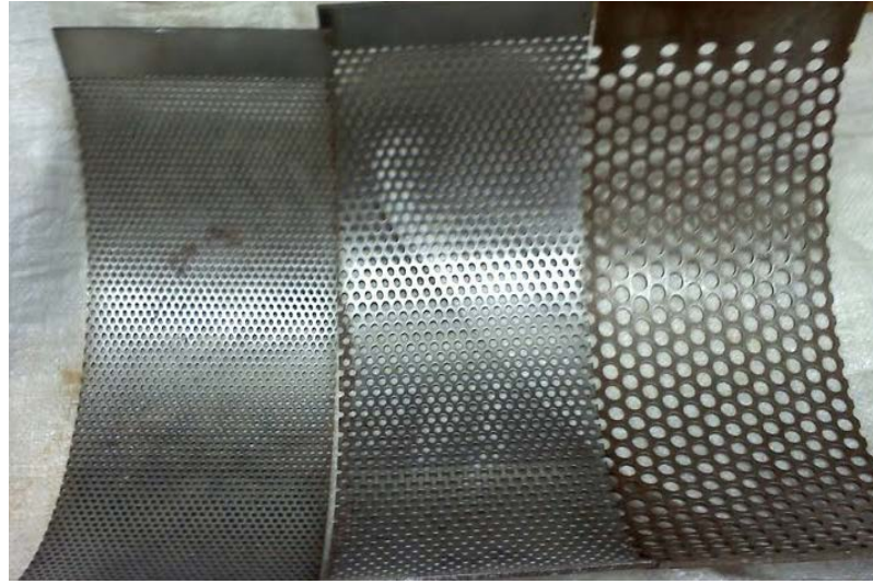
Figure 3-1 Different Screen Sizes used in the Hammer Mill (from left to right 3 mm, 5mm, and 10 mm)
