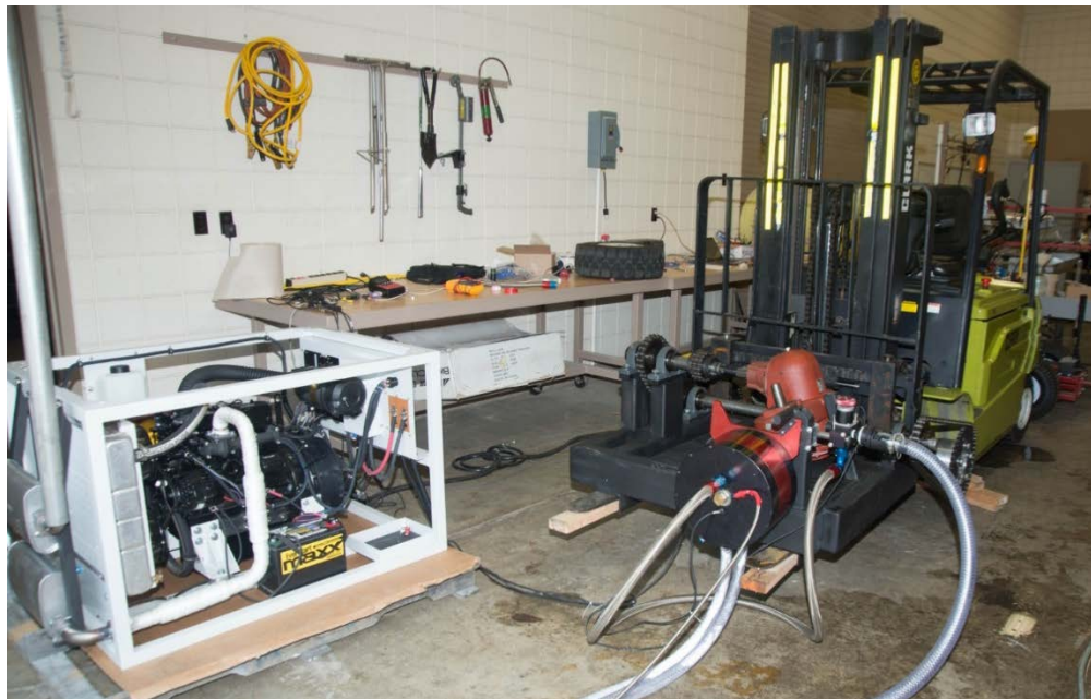
Figure 3.2 Hybrid drivetrain set up for testing. Polar power generator (left) and forklift frame connected to dynamometer (right).
