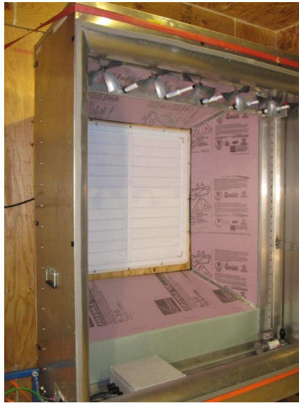
Figure 4-10 – Fan testing setup; treatment 36_54_60I
