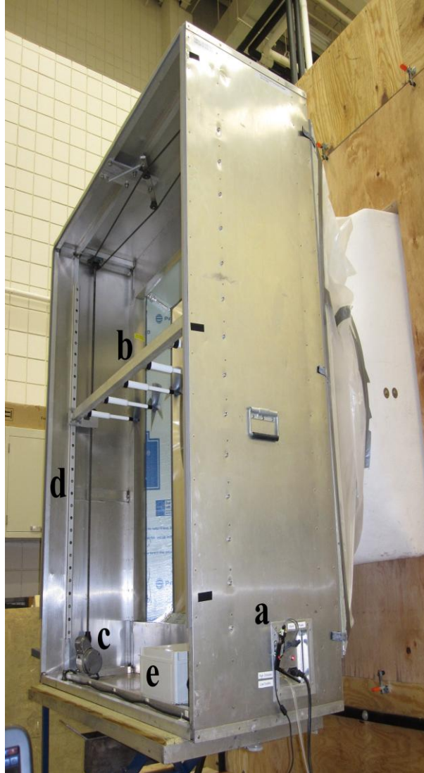
Figure 2-1 – FANS unit; a) interface panel, b) anemometer array, c) electric motor, d) vertical guide rail
