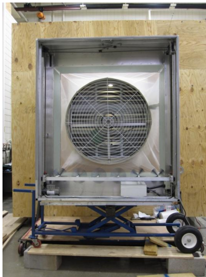
Figure 4-23 – Fan testing setup; treatment 48_54_60D
