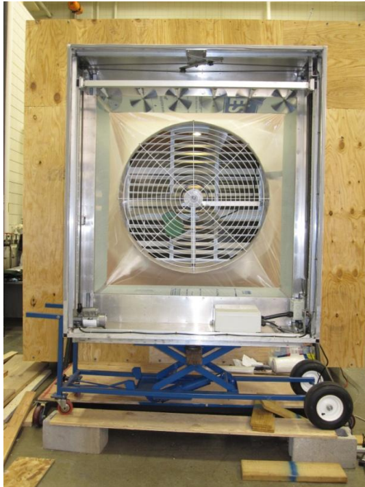
Figure 4-22 – Fan testing setup; treatment 48_54_45D
