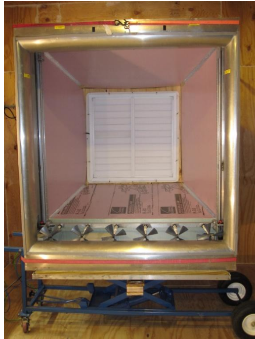
Figure 4-8 – Fan testing setup; treatment 36_54_30I
