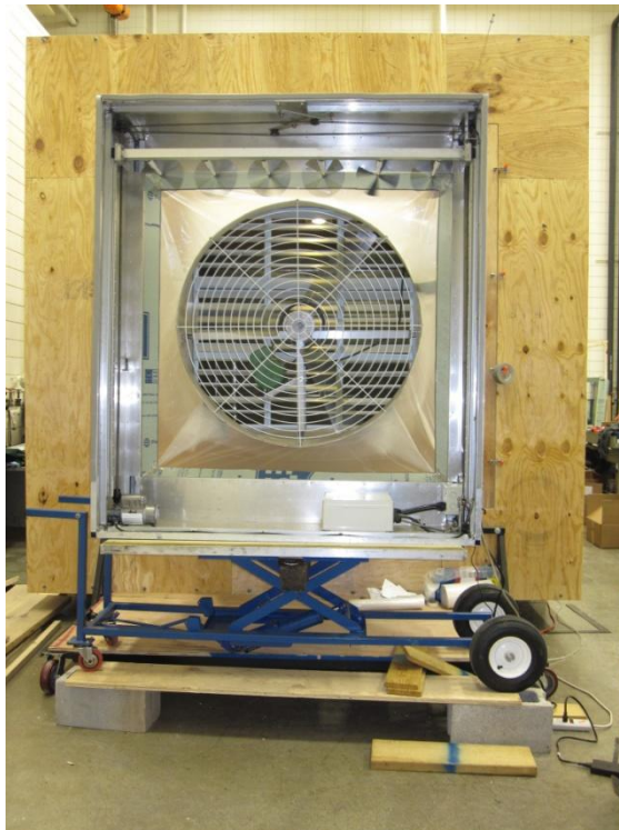
Figure 4-21 _ Fan testing; Treatment 48_54_30D
