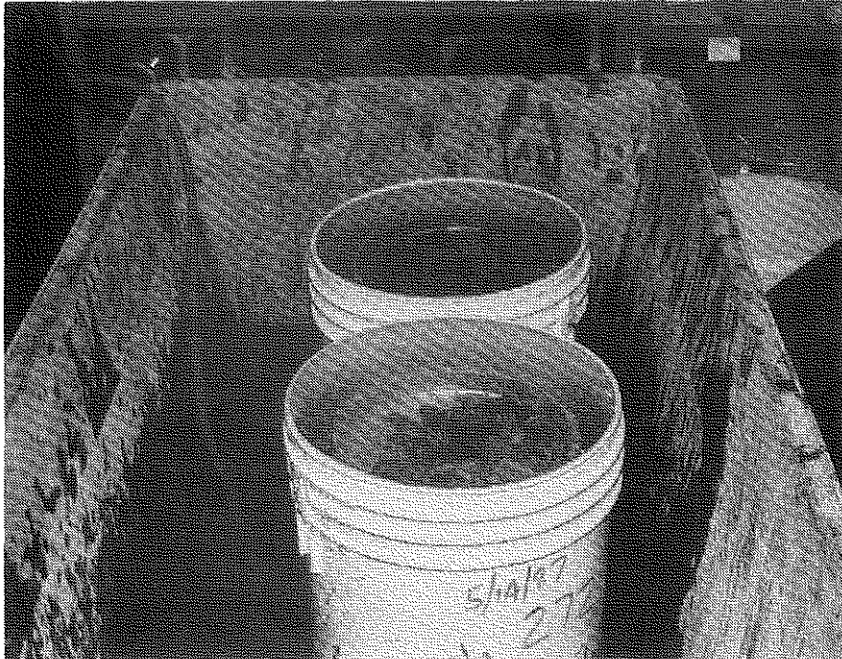
Figure 3. Aggregate Samples being Washed Free of Sodium Sulfate Solution.
