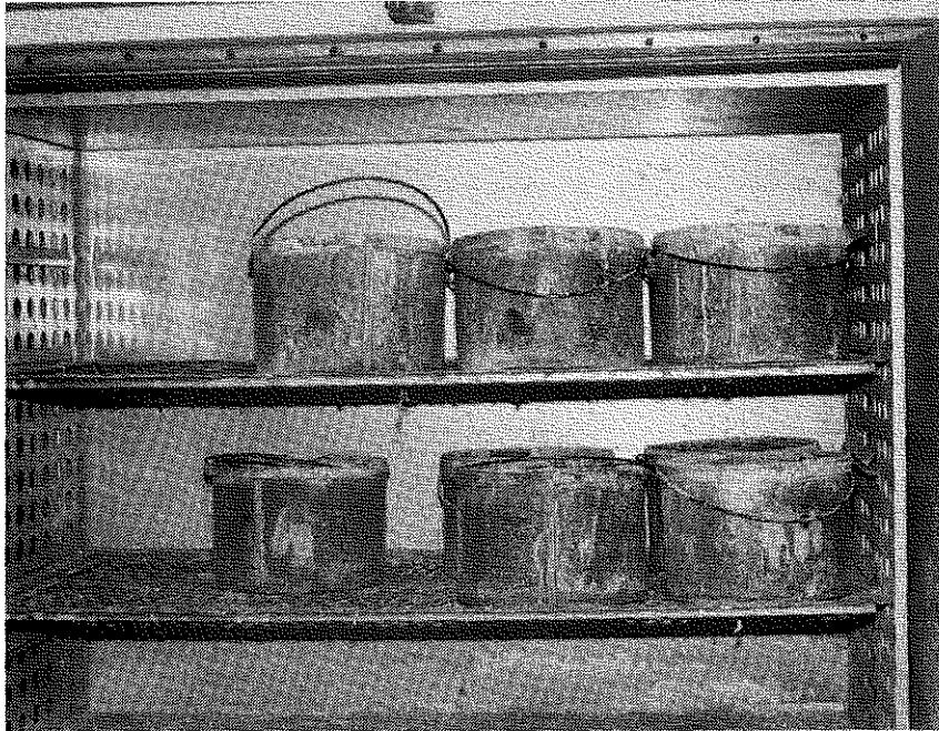
Figure 6. Aggregate Samples in Drying Oven at the Division of Materials' Laboratory.
