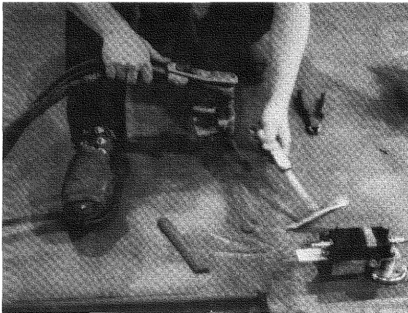
Figure 12. Welder Chipping Flux during Welding Operation.
