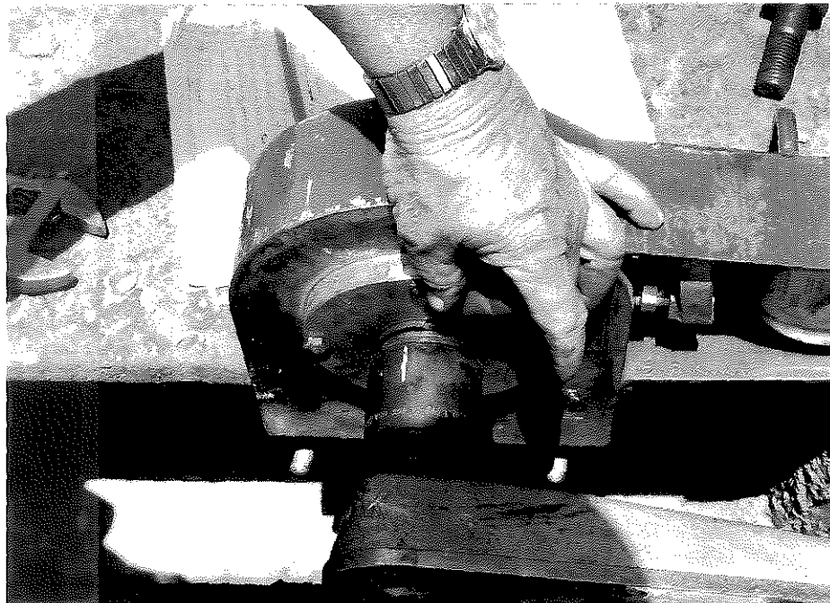
Figure 2. A Feeler Gage Inserted into the Gap of a LIW Being Tested on a Skidmore-Whilhelm Bolt Tension Calibrator.
