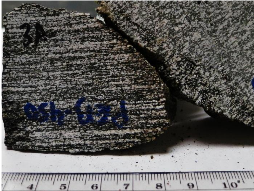
Figure 7.7. Cut sample of Monson amphibolite showing mineral lineation defined by hornblende needles and feldspar streaks. Left face is perpendicular to foliation and parallel to lineation. Right face is perpendicular to lineation.
