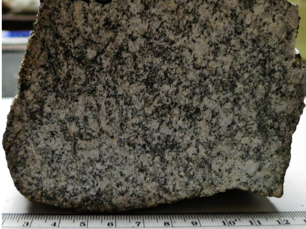
Figure 5.7. Sawn slab of typical appearance of unfoliated, medium grained Hardwick biotite hornblende tonalite.
