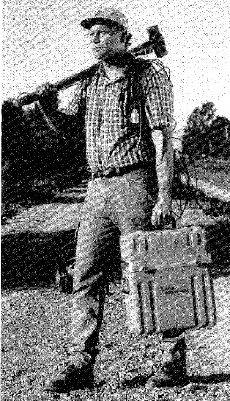
Figure 4. Typical Equipment Used on Site Investigations: Seismograph, Geophones, and Sledgehammer.
