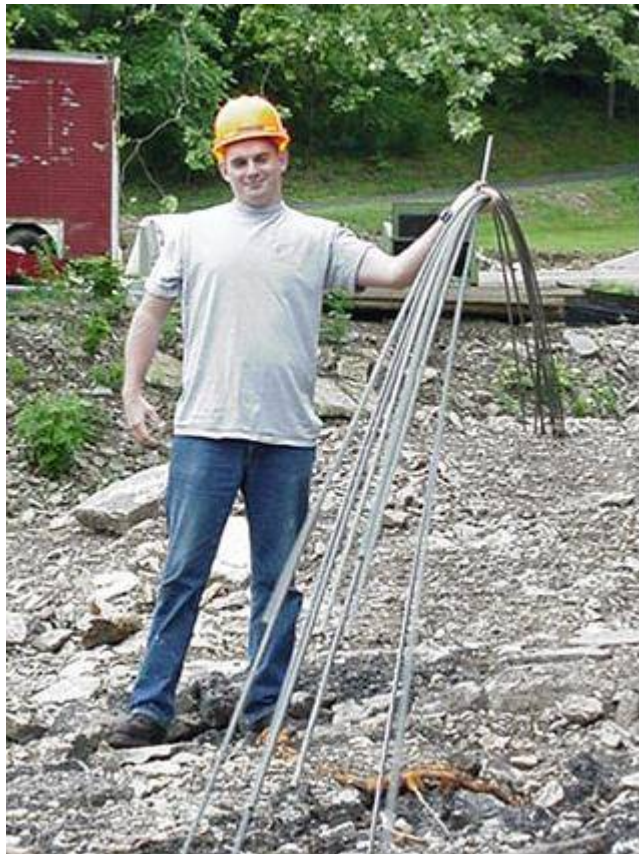
Fig. 3.1 – Light-weight CFRP bars.
