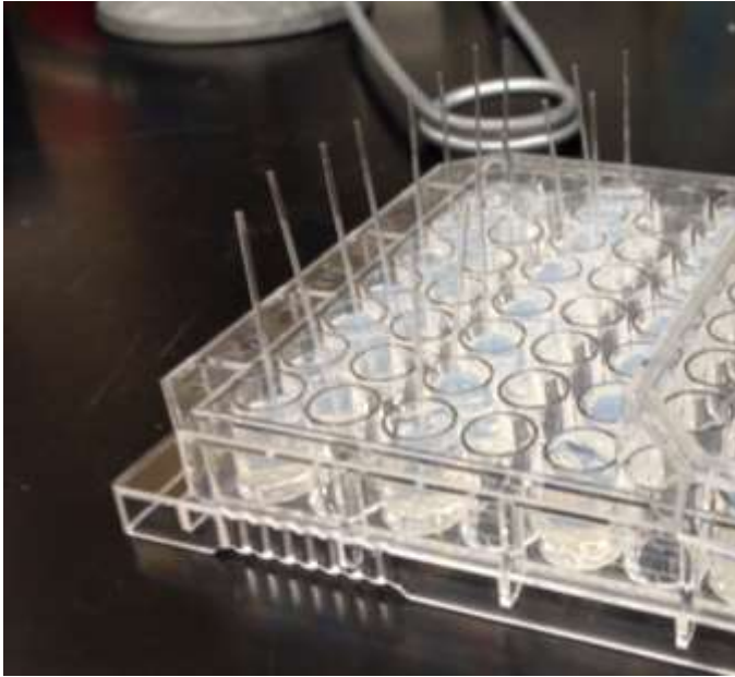
Figure B.3 Chemotaxis setup - plate with inserted capillaries after sealing over the flame.
