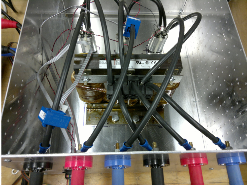
Figure A.9: Three-phase inverter output LC filter
