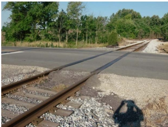
2013 After replacing the Rubber/Asphalt Surface
