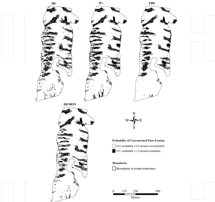
Figure 8. Discretized erosion probability maps for the logistic regression analysis of the RTK dataset comparing the D8, D_{\infty} , FD8, and DEMON flow direction algorithm.
