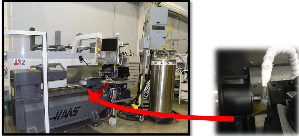
Figure 3-1. Experimental setup for cryogenic machining on HAAS TL-2 CNC lathe. Right hand side detail of cryogenic cooling during a facing cut shows how liquid nitrogen is applied onto the rake face of the cutting tool through a 3mm diameter nozzle. The process displayed is face turning, during which the cutting tool traverses radially inward.
