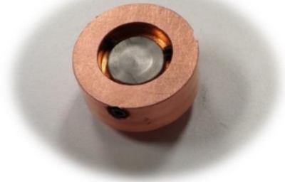
Figure 3-8. Hitachi S4300 scanning electron microscope and custom copper sample holder for machined porous tungsten samples. The holder substantially improved image quality by draining electrical charge efficiently.
