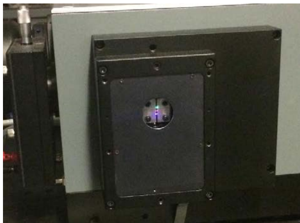
Figure 6-10 Alignment diodes imaged on the entrance slit of the spectrometer
