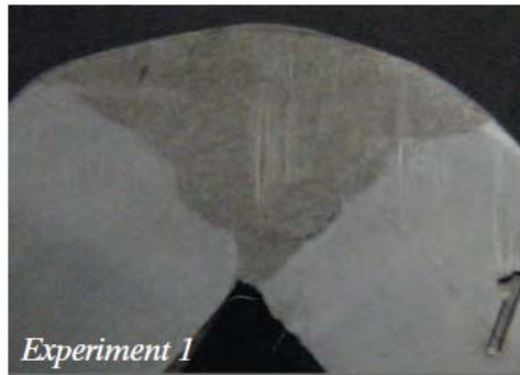
Figure 3 Cross-section of weld made by non-consumable DE-GMAW using plasma bypass arc. I_{bp} = 100 A, I_{bm} = 145 A [17].
