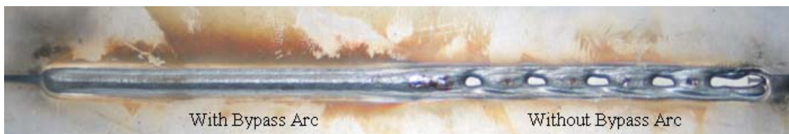
Figure 8 Comparison of weld on lap joint made by controlled DE-GMAW and conventional GMAW process [18].
