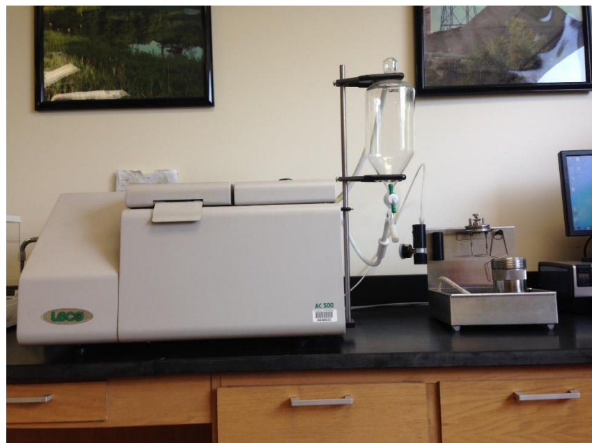
Figure 6.3. LECO AC500 calorimeter
