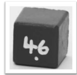
Figure 4.5. A 1.46 SG density tracer block.
