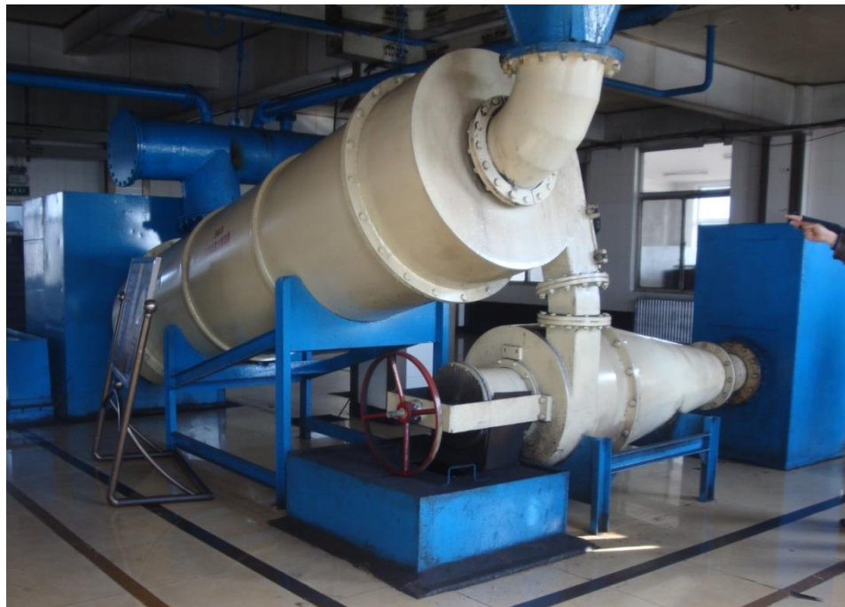
Figure 2.1. Schematic illustration (top) and picture (bottom) of the gravity-fed 3-product H.M. cyclone.
