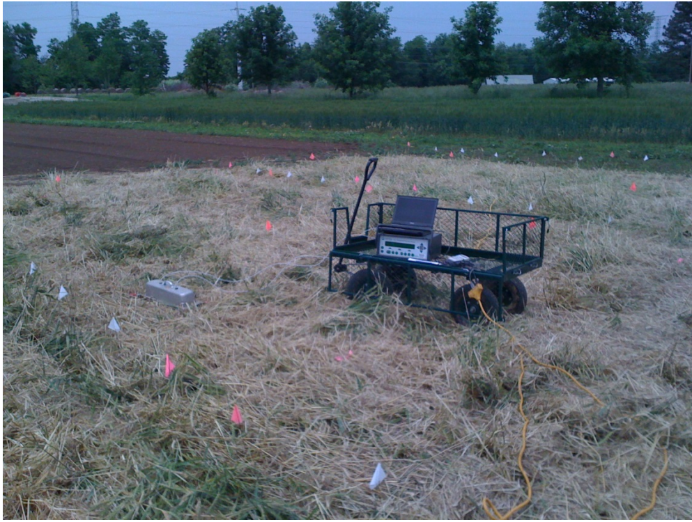
Figure 2.6: Field measurements of gaseous emissions taken using the static chamber method and a photoacoustic spectroscopy gas analyzer.
