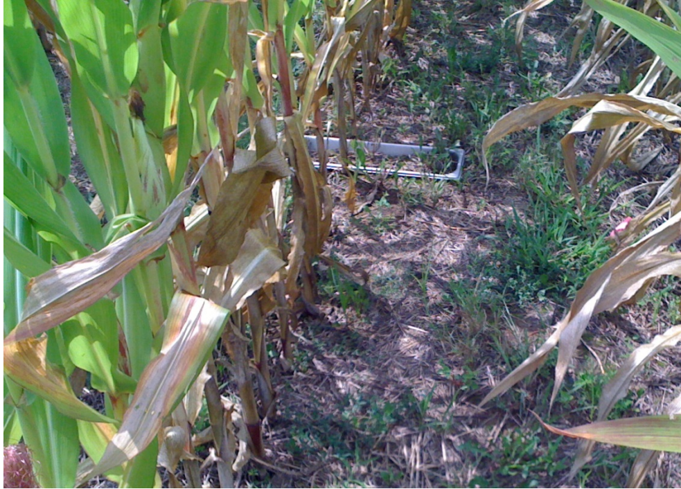
Figure 2.5: Trace gas pan placed between corn plants and spanning soil surface area both within and between rows.
