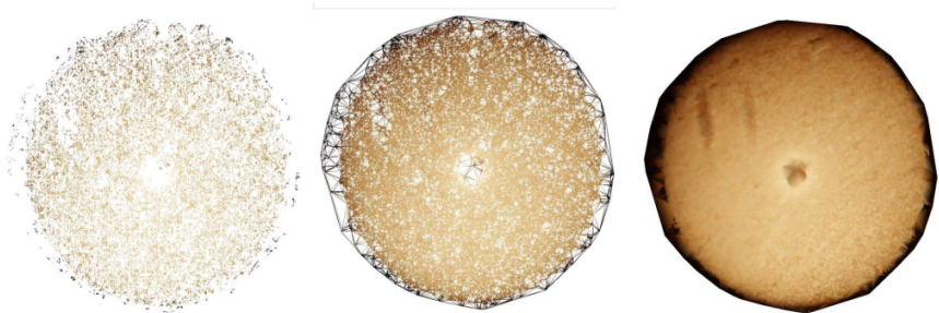
Surface Triangulation of the point cloud.
