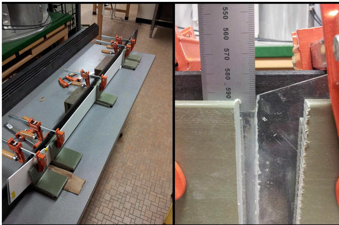
Figure 2.22: Left: The full light guide gluing jig. The plastic ‘L’ pieces are used to clamp the scintillator and light guide pieces in place. By using the same ‘L’ pieces at all clamping points, we maintained an even spacing between the plastic and the back wall, which is necessary to achieve a solid glue joint. Right: A close up of a single glue joint. The overhang is 9 mm for all joints on the interior angle side of the joint. This joint is both structural and for the light transmission, as the optical cement matches the index of refraction of the light guides.
