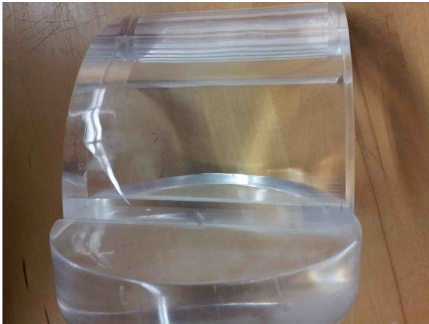
Figure 2.20: The same arc as in Figure 2.19 , but after undergoing the full polishing process we developed. The mirror finish and overall transparency are in the final, acceptable state.
