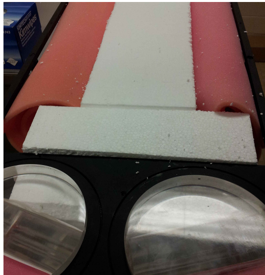
Figure 2.28: Photograph of detector during final assembly, after inserting foam. The foam acts as a shock absorber for the entire system, as well as to help hold the plastic in place.
