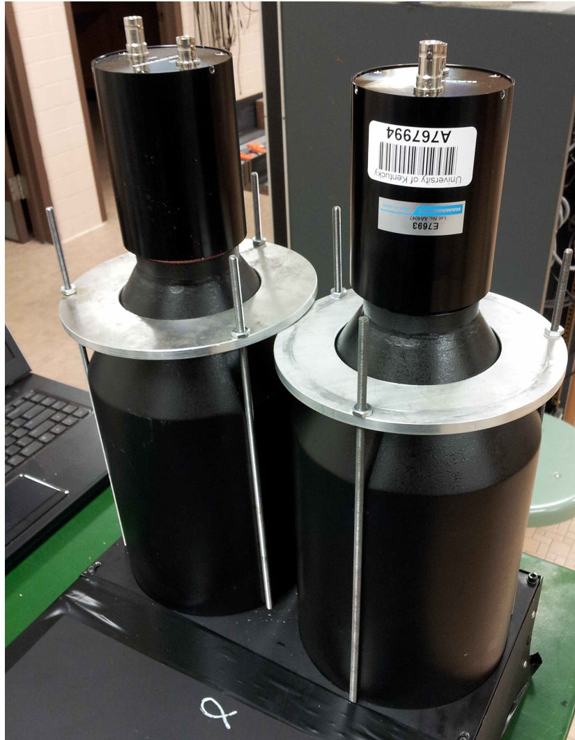
Figure 2.30: Photograph of detector during final assembly, PMT mounting system. The black pieces are mu-metal shields designed to stop magnetic effects from interfering with the PMT function. The aluminum collars are designed to seat onto necks of the mu-metal shields and clamp them in place. The PMTs are seated tightly into the mu-metal shields using foam. This whole assembly holds the PMTs tightly against the cylindrical light guides to obtain a solid optical connection.
