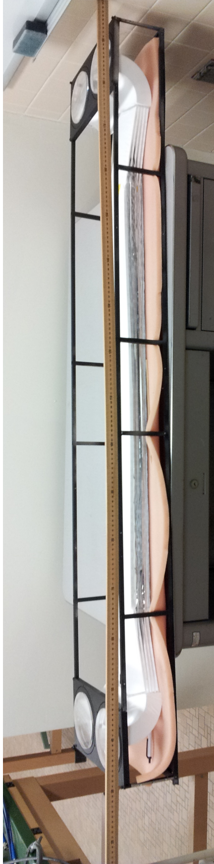
Figure 2.21: The aluminum frame which will house the detector. The detector pieces are sitting inside, loosely fitted to check sizing. The cylindrical gaps on the end caps are pass-throughs that allows the cylindrical light guides to reach the PMTs which will be mounted on the outside of the frame.
