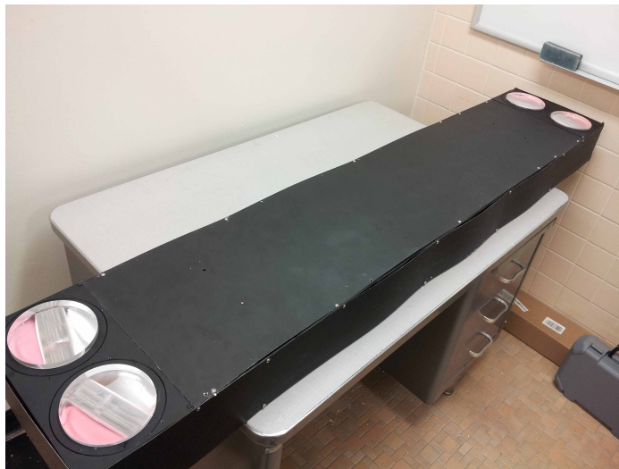
Figure 2.29: Photograph of detector during final assembly, after attaching outer aluminum skin. The skin seals out light as well as adding rigidity to the entire design. By fastening the skin in place at many locations, the skin is rigid against flexing in it's wide dimensions.
