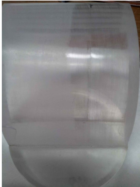
Figure 2.19: A light guide arc after manufacture. On the left is the raw surface, on the right is the surface after a buffing wheel has been passed over. On the left, the surface is extremely cloudy and there are cuts and abrasions in the surface that must be removed. On the right, the abrasions remain after light surface treatment, necessitating a more rigorous treatment.
