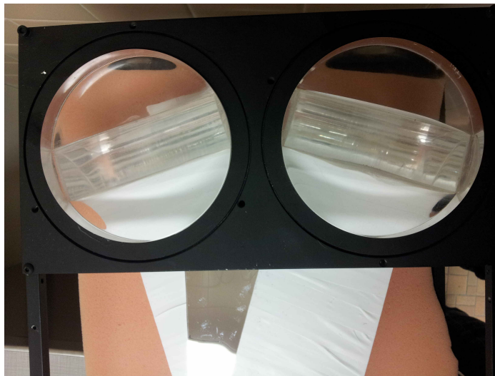
Figure 2.27: Photograph of detector during final assembly, end cap. The pass-through allows light from the layers to interface with the PMTs (not attached yet). The unique 'Y' design to separate light from adjacent layers is demonstrated.
