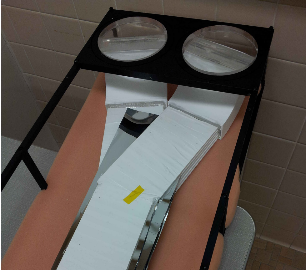
Figure 2.26: Photograph of detector during final assembly, without foam. The reflective sheets are aluminized Mylar, meant to optically isolate the scintillation layers.
