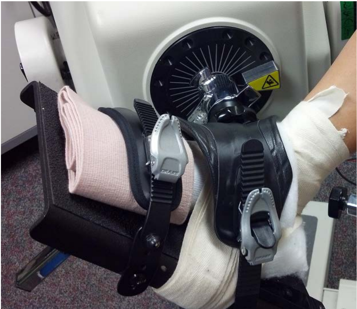
Figure 4.1: Setup of the foot on the Biodex dynamometer.
