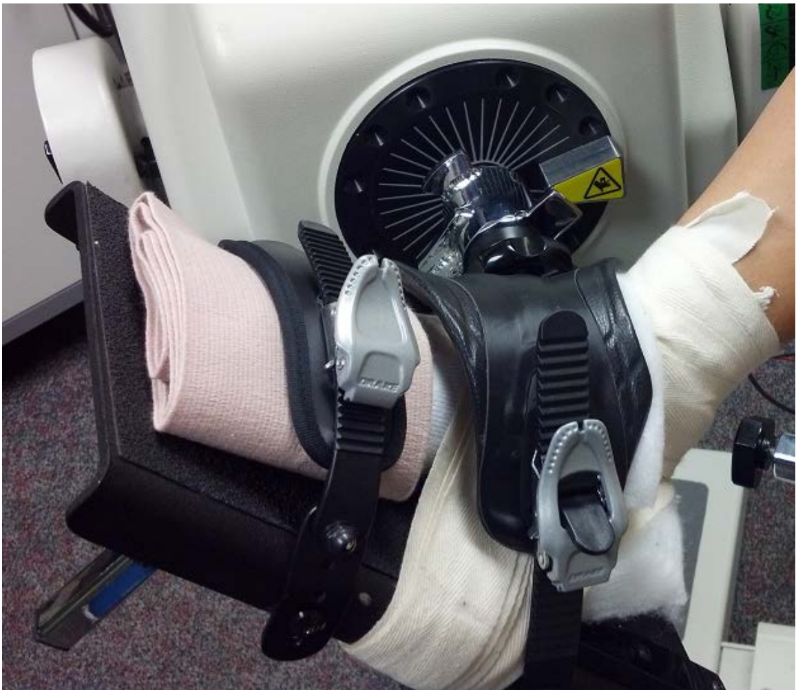
Figure 3.1: Setup of the foot on the Biodex dynamometer.
