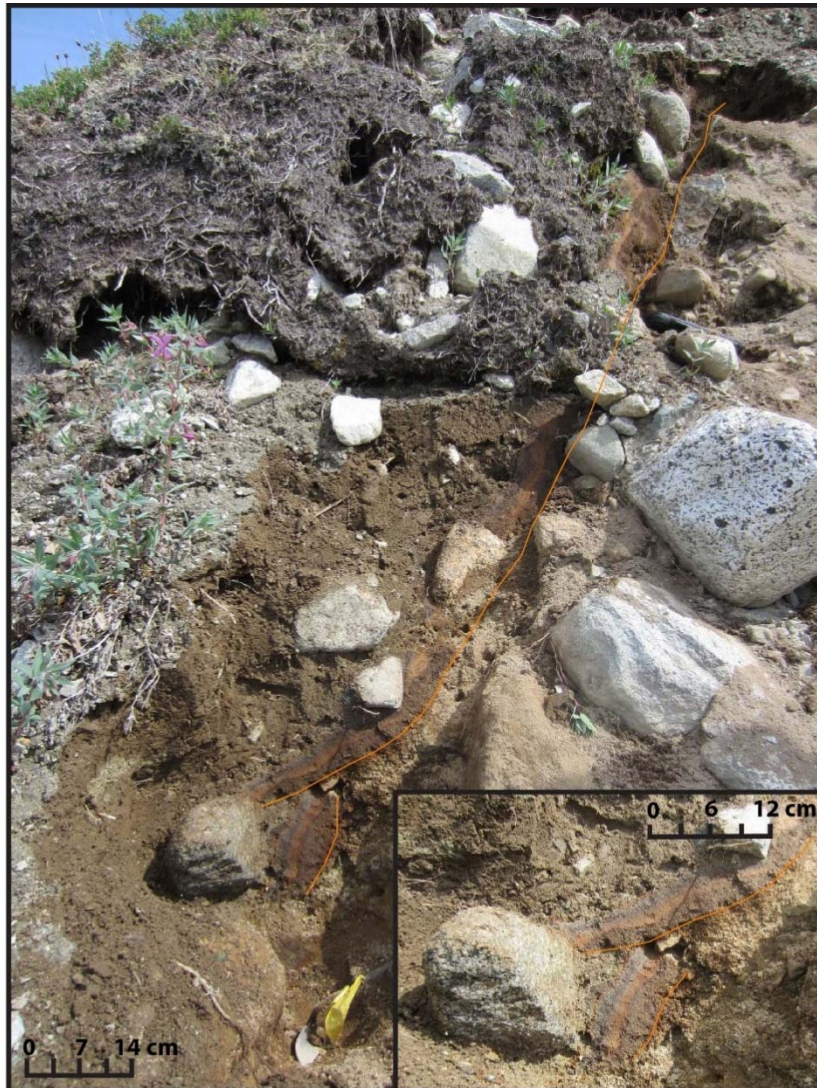
Figure 4.6: Cross-section of the Slippery Creek scarp. A continuous layers of organics and clays are bulldozed in a common blind thrust style with an offset of the continuous layers occurring in line with the base of the scarp. A blowup of the offset is shown to the right. The orange lines follow the bottom of the organic and clay layers.
