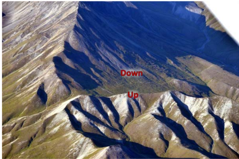
Figure 4.7: Southern East Fork fault. View to the southeast towards the Denali fault. The south-side down displacement shown in the image of the East Fork faults oppose the south-side-up topographic expression of the foothills. The bottom image is a zoomed in image of the fault and the fault can be seen clear by the offset shadow in the bedrock. The red line traces the fault trace. The down and up labels just show relative motion.
