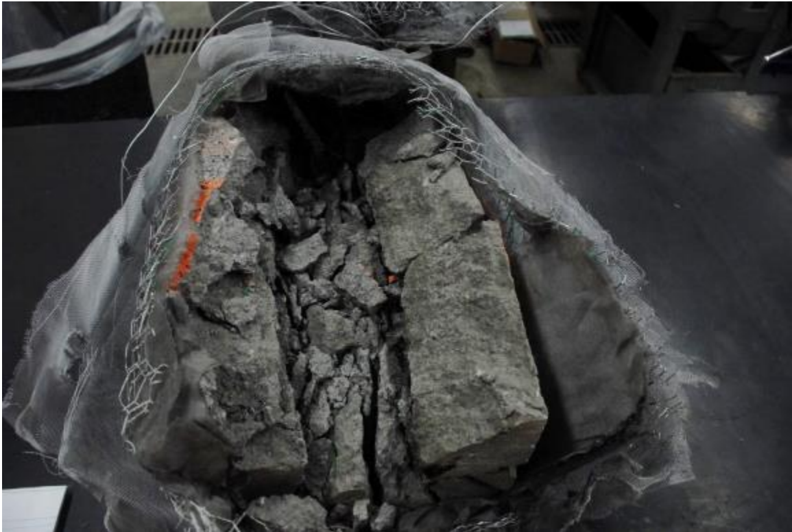
Figure 4-9: Small fragments centered around the blast hole
