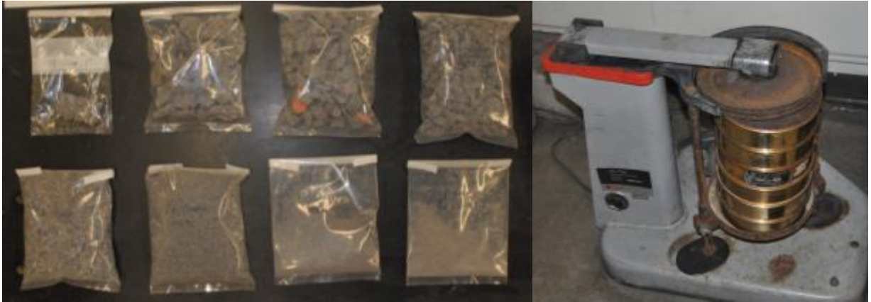
Figure 4-10: Small size sieve analysis
