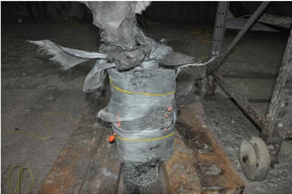
Figure 4-5: Contained fragments after detonation
