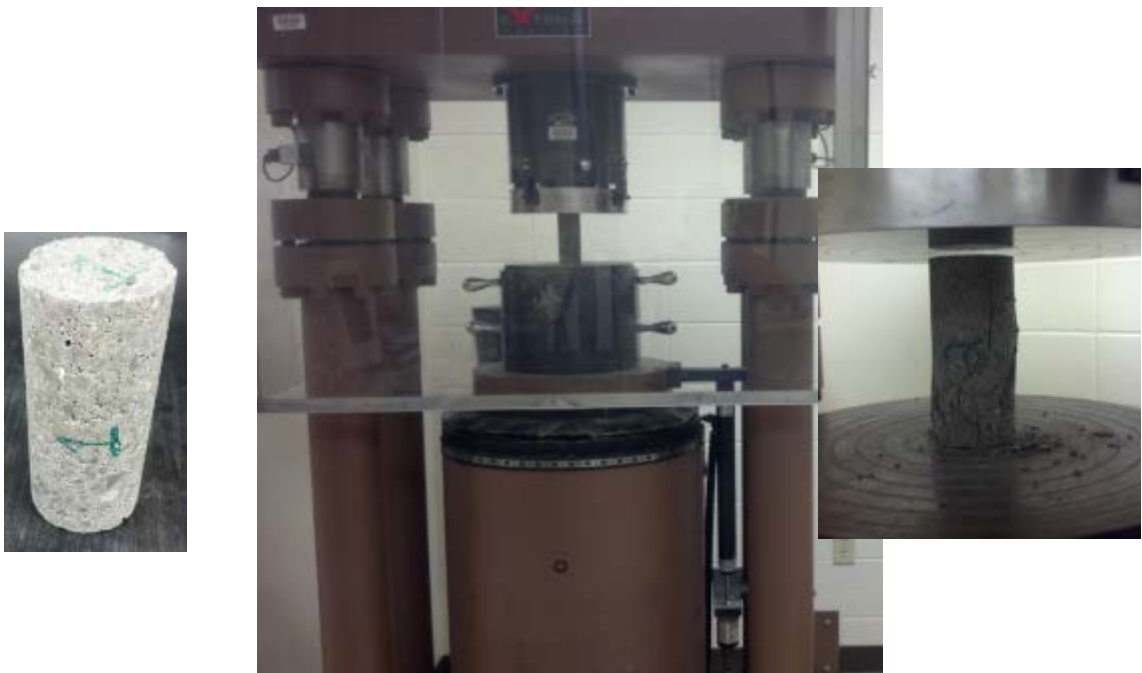
Figure 5-2: Testing Machine and inserted core sample
