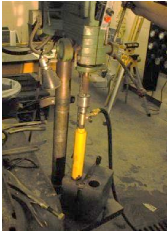
Figure 5-1: Concrete blocks being cored
