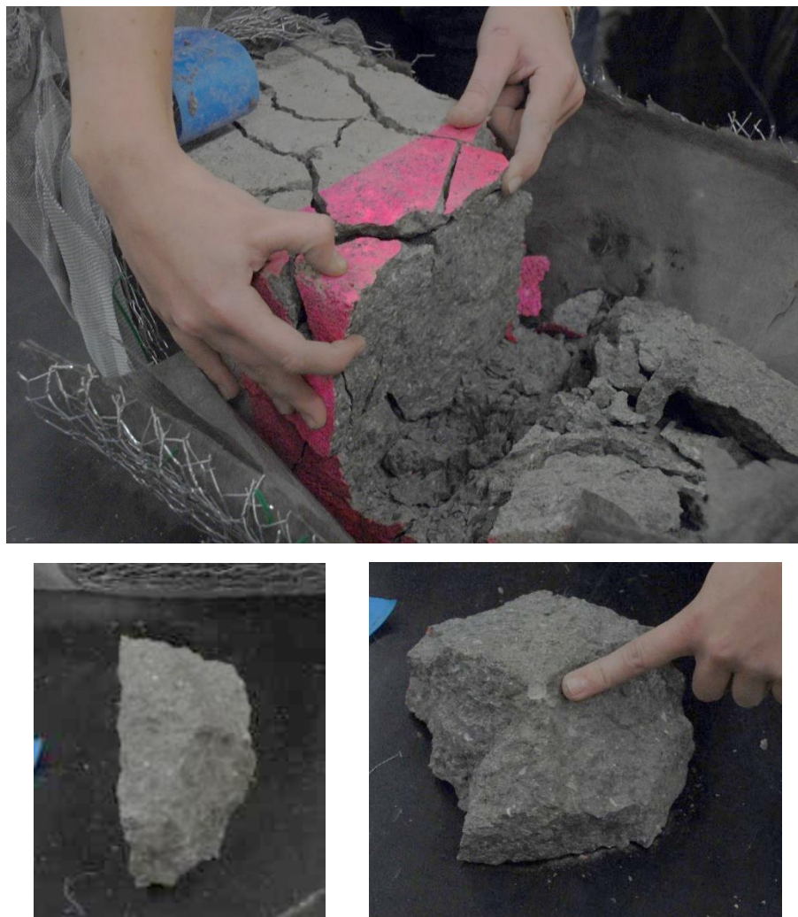
Figure 4-21: Top: straight crack through the center of T3c; Bottom: large fragment from the center of the block
