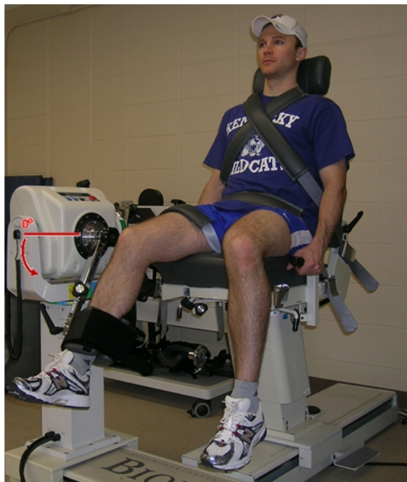
Figure 4.1. Dynamometer testing setup. Included are the BIODEX test chair, right knee attachment, as well as, chest, waist, thigh and tibia stabilization straps.
