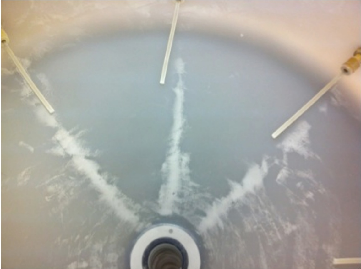
Figure 3.5: Photograph of the inside surface of the conical section of drying column showing polymer blend particles settled on its surface.
