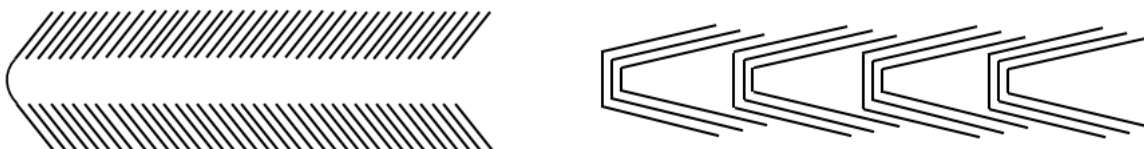
Figure 6. 5 Schematic representation of herringbone MWCNTs and nesting cup (bamboo) MWCNTs.
