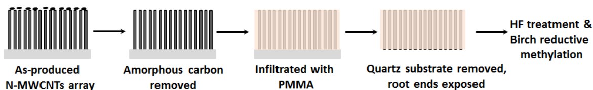
Figure 7. 15 Schematic illustration of the key steps involved in infiltration of polymer into interstitial spaces between N-MWCNTs in the array and exposing bottom ends of the tubes to performed chemistry alone. 88
