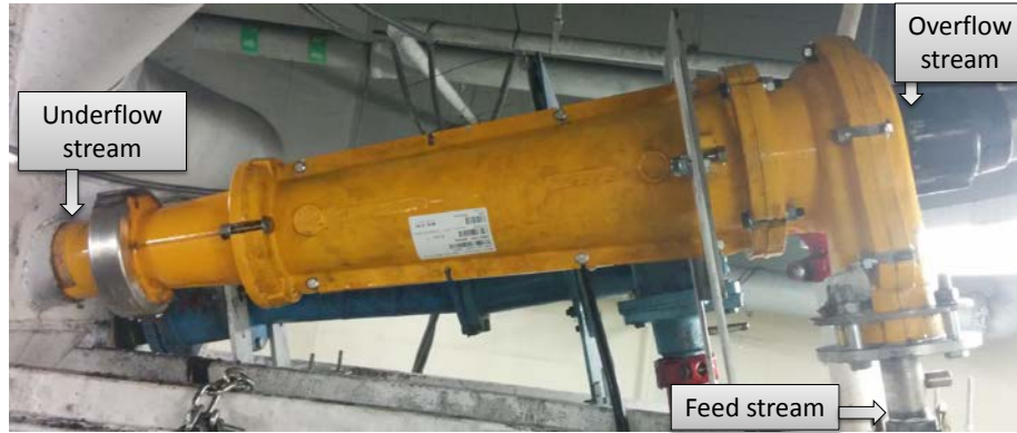
Figure 4.7: Dense medium cyclone with 15–cm diameter used in the experimental test program.
