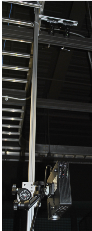
Figure 3.5: Projector Holding System
