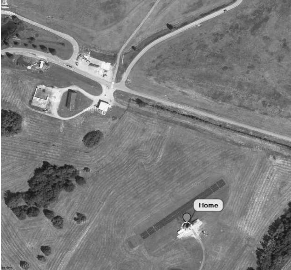
Figure 7.1: Lexington Model Airplane Club . Shown is a screenshot from the Mission Planner software. The Lexington Model Airplane Club field is located on the east side of Lexington, KY. The field features a 200 meter runway oriented WSW and ENE. The “Home” label indicates the GPS coordinates where the Ardupilot calibrates its zero altitude.
