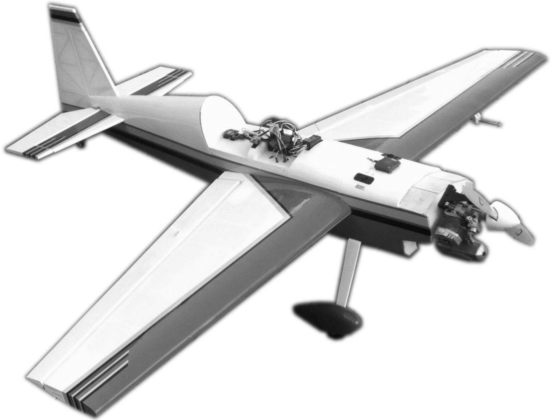
Figure 4.1: The AeroWorks EDGE 540T . The EDGE is a mid-winged, aerobatic, remote-controlled aircraft with a 1.52 m wingspan.
