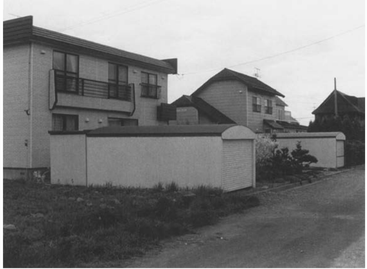
56. Houses in Tomakomai, Hokkaido. The climate here is analogous to that of New England. The roadside garages, which are connected to the houses, obviate snow removal from the private driveways during the winter. Note, also, the absence of lawns. Originally settled by colonist militia (Tondenhei) in the late nineteenth century, Tomakomai is a prosperous industrial city of more than 160,000. It is the leading producer of paper in Japan. Oil refineries and aluminum and lumber plants are also located here.
