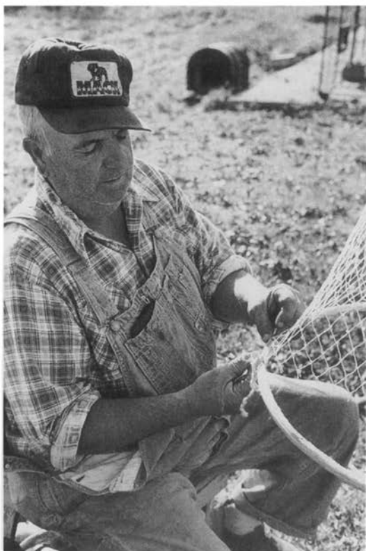
Orval Loven fastening webbing to the hoop on a hoop net, Grayville, Illinois, 1977.
