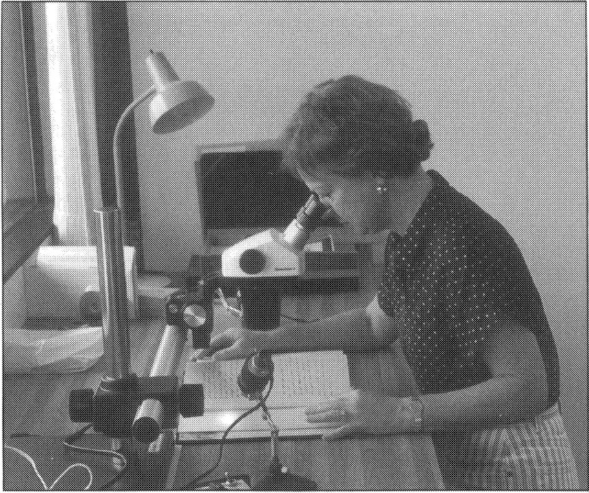
Figure 5.8. The stereomicroscope is the document examiner's basic instrument. Here Maureen Casey Owens, who for twenty-five years was the Chicago Police Department's questioned document expert, uses the binocular instrument to examine the handwriting of the purported Jack the Ripper diary.
