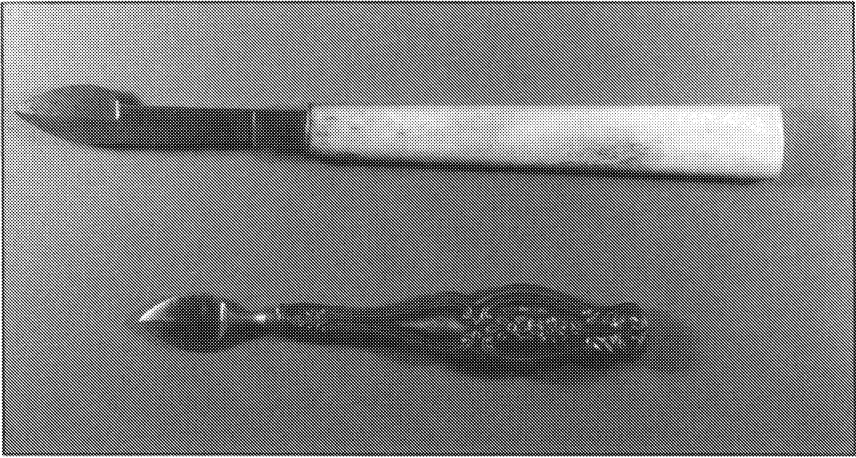
Figure 4.9. Ink-eraser knives (like the bone-handled and sterling silver models shown here) were used throughout the dip-pen era to scrape mistakes from parchment or (with more care) from paper. Such erasures are, naturally, easily detected.
