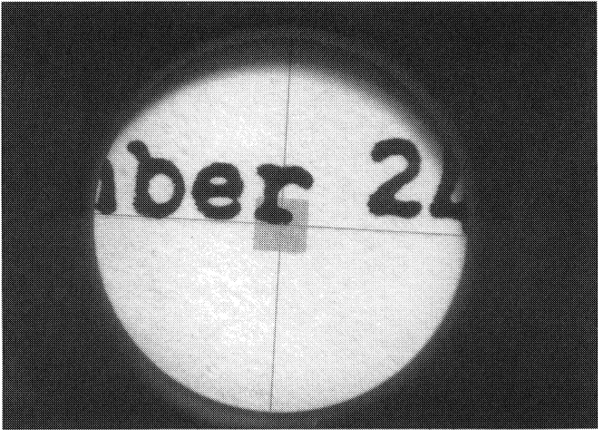
Figure 2.14. Detail from one of the MJ-12 documents reveals that the date numerals are out of alignment with the other characters, indicating that the numbers were typed at a different time.
