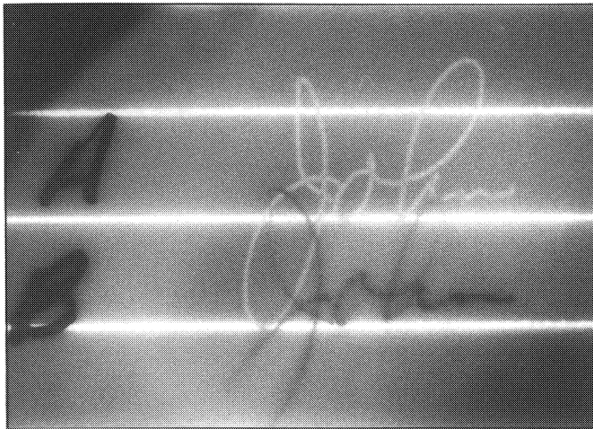
Figures 6.4 and 6.5. Two common black inks are indistinguishable by the unaided eye (above) but appear quite different when an infrared luminescence analysis is conducted (below). Photos courtesy of John Fischer.
