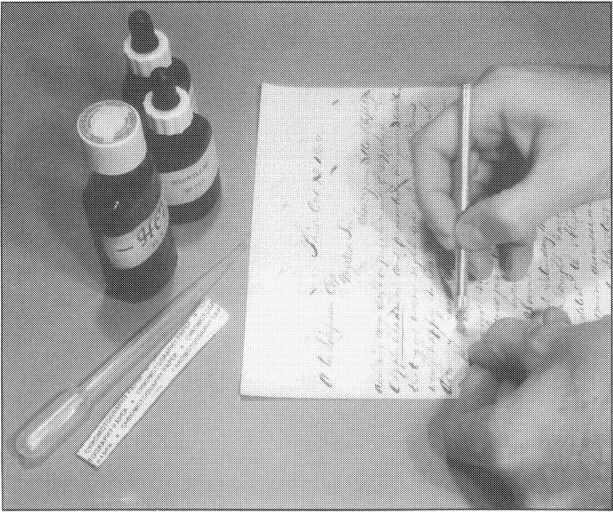
Figure 7.1. A tiny amount of ink from a document is carefully transferred to a strip of special laboratory paper. “Spot tests” (based on the reaction to a drop of reagent) can then be performed without harming the document.
