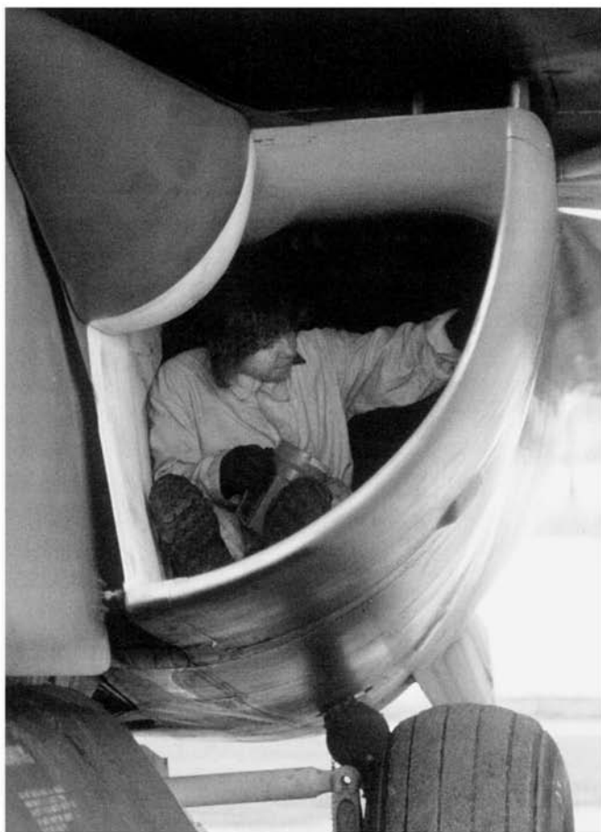
A ground crew chief inspects the intake of an F-111A aircraft. Courtesy of the U.S. Defense Visual Information Center.
