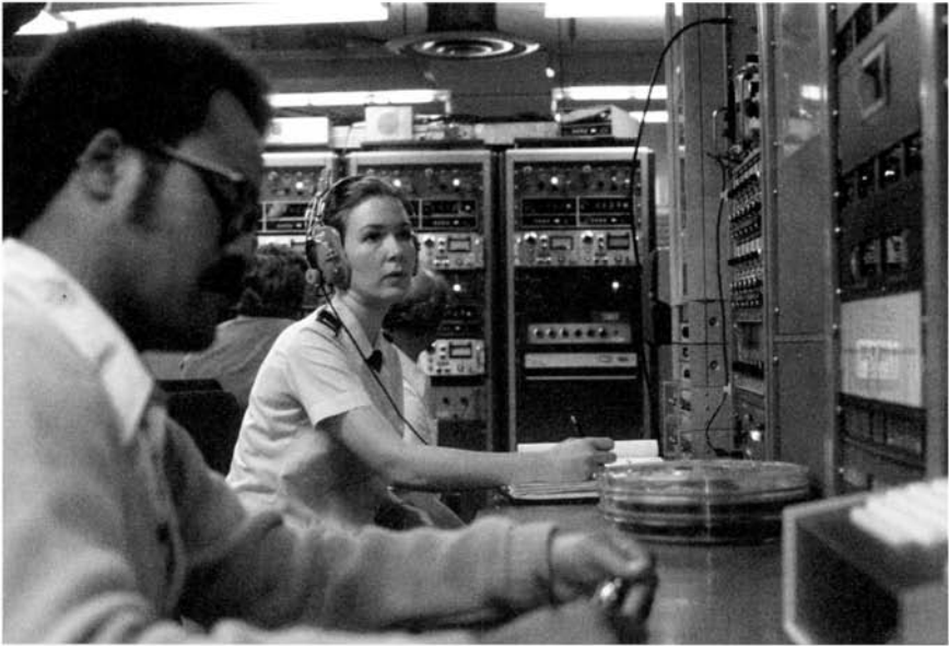
Captain Mary Collier is an aircraft structural engineer for the Air Force. She is listening for stress cracks in the wings of an F-111 aircraft. Courtesy of the U.S. Defense Visual Information Center.
