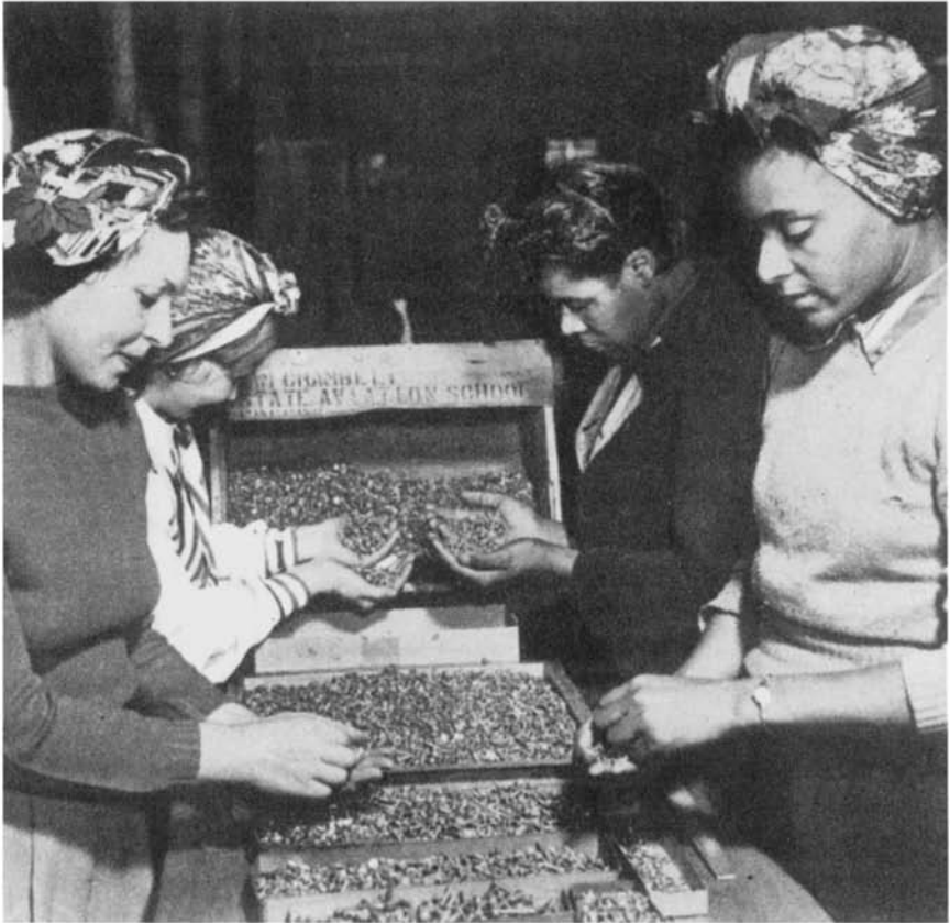
Sorting rivets by size was the job of many female aircraft workers. Courtesy of the General Motors Corporation.
