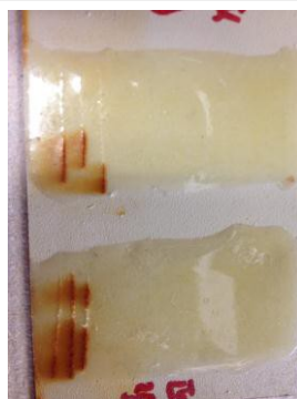
Figure 10—Polyurethane films after salt water bath; without microcapsules (left) and with microcapsules (right).
