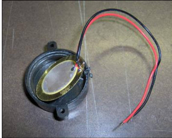
Figure 3.5 – Piezo Element Separated from Casing
