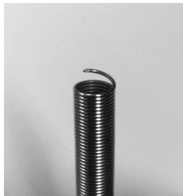
Figure 2.2 – Small Cluster Spring: Cut End
