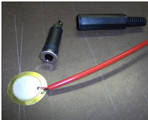
Figure 3.6 – Piezo Element and 1/4" Jack
