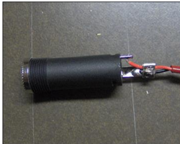
Figure 3.8 – 1/4" Jack: Wires Soldered, Tabs Bent
