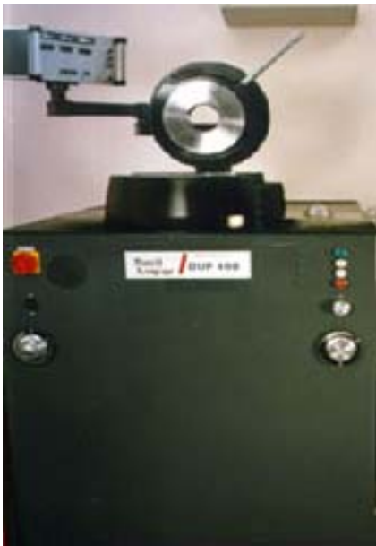
Figure 3- 2 Tinius-Olsen BUP 200 Ductomatic sheet metal testing machine
