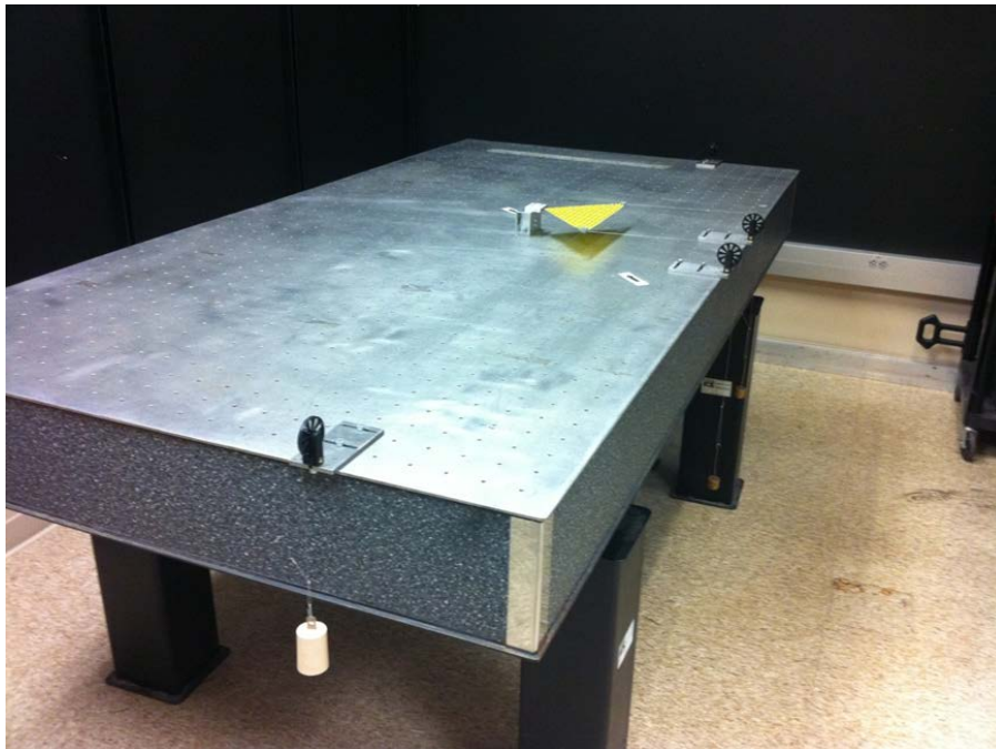
Figure 3.1. Experimental set up for photogrammetry experiments measuring static deflection of coated nylon fabric.
