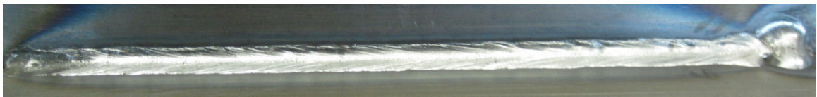
Fig. 7.7 Weld Bead of Conventional SAW Experiment (Direction: R to L)
