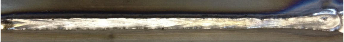
Fig. 4.8 Weld Bead in “Large-Root opening” Experiment (Direction: Right to Left)
