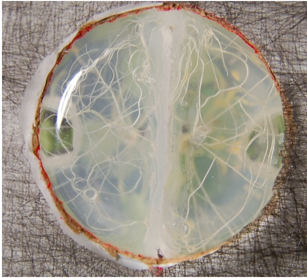
Figure 2.2: Bottom-Up View of a Barrier Pot with Growing Plant Roots & Visible Wells
