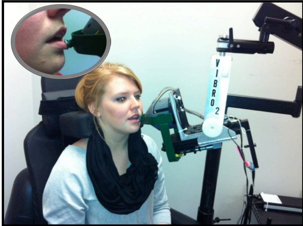
Figure 4: Vibrotactile Mechanical Stimulus Delivery System Setup and Subject Orientation.
