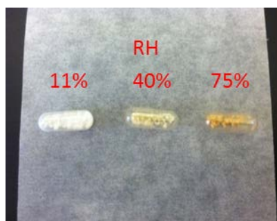
Figure 6.5. Photograph of capsules of SD pure tobramycin stored at three different RH % and 40°C for 2 weeks.
