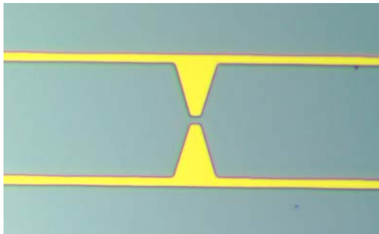
Figure 4.4 - Picture of Fabricated Bowtie with Full Coplanar Line Separation
