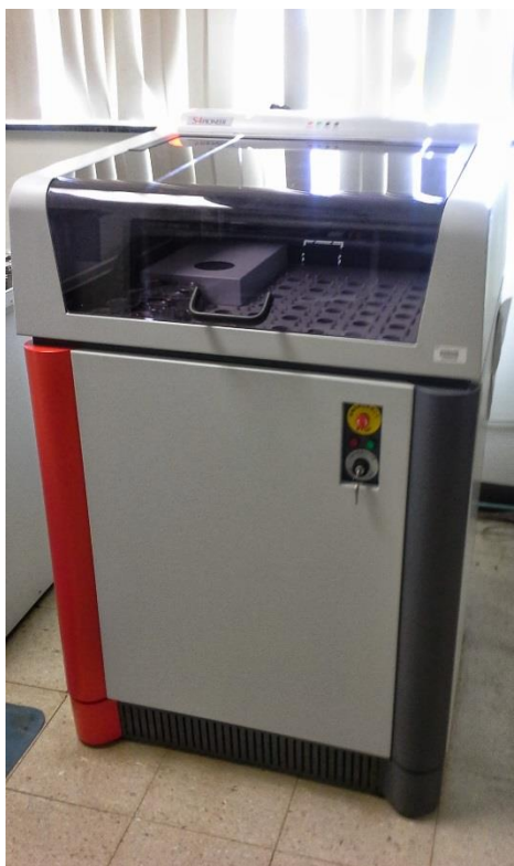
Figure 3.3. S4 pioneer-wavelength dispersive X-ray fluorescence spectrometer
