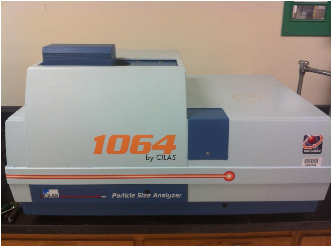
Figure 3.1. CILAS 1064 particle size analyzer
