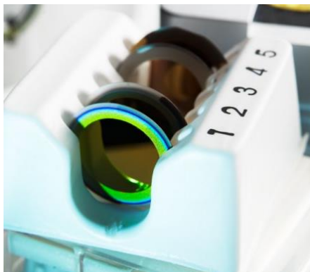
Figure 2.7. Picture of QCM-D sensor (q-sense.com)
