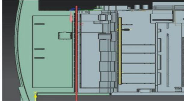
Figure 42: Top view of the Meander Antenna (yellow line) location with respect to the paper path (red line)
