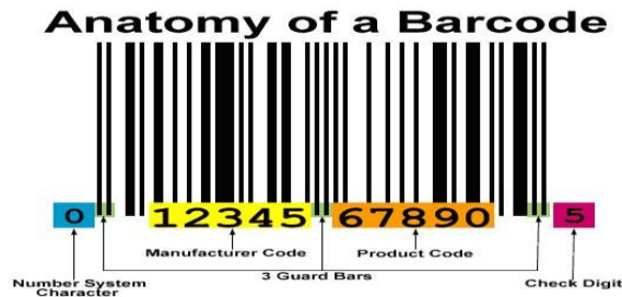
Figure 2: Anatomy of a Bar Code
