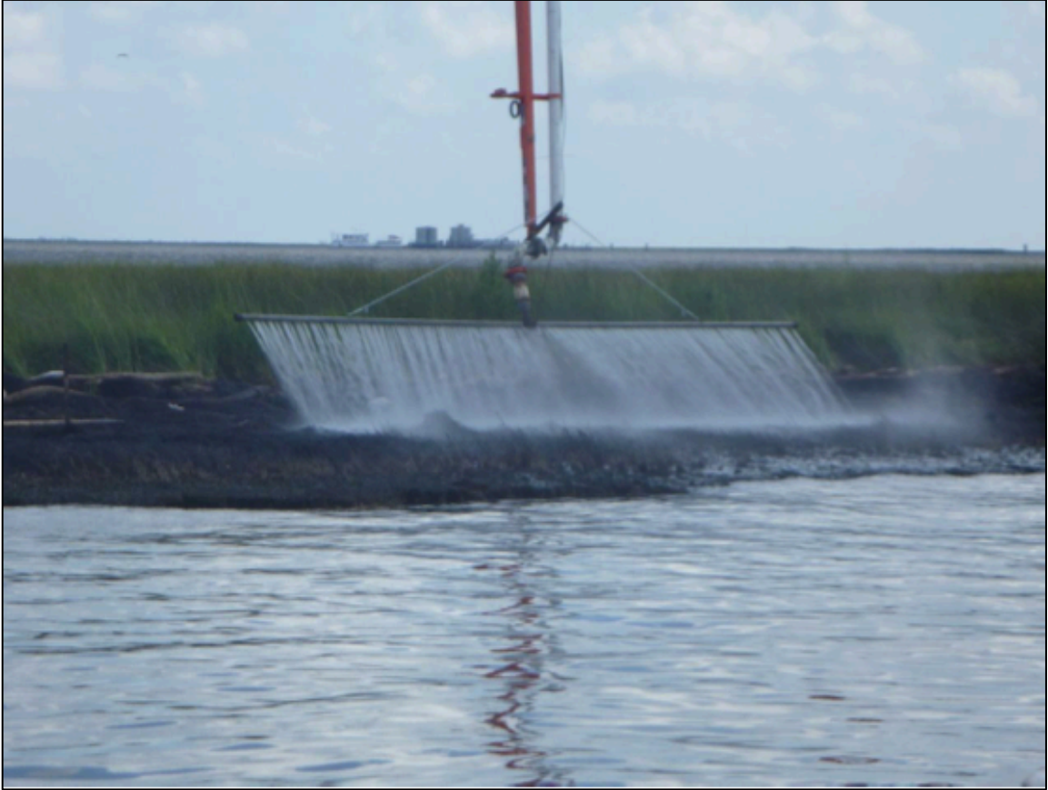
Figure 2.7. Photograph of low pressure, high volume marsh flushing tested at Bay Jimmy, LA in September 2010. NOAA reports indicate that little to no oil was effectively mobilized from the sediment during demonstrations, and the flushing may have actually damaged the marsh by scouring sediments (Zengel and Michel, 2013). However, following vegetation cutting, this remediation method was approved for use at DBI and other sites.
